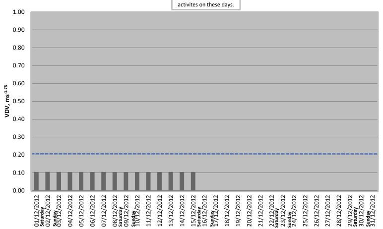
A transfer function equivalent to doubling the night-time VDV measurements has been applied to obtain values representative of an upstairs, mid-floor receptor location. VDV threshold for Education establishments, offices and similar is 0.40ms<sup>-1.75</sup> and Commercial is 0.80ms<sup>-1.75</sup>. Therefore it may be necessary to adjust the threshold displayed on the graph if buildings other than residential dwellings are being assessed.
