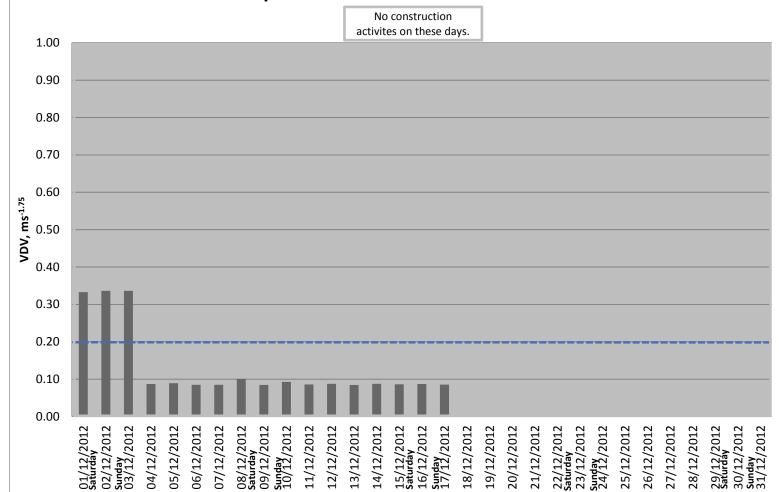
A transfer function equivalent to doubling the night-time VDV measurements has been applied to obtain values representative of an upstairs, mid-floor receptor location. VDV threshold for Education establishments, offices and similar is 0.40ms<sup>-1.75</sup> and Commercial is 0.80ms<sup>-1.75</sup>. Therefore it may be necessary to adjust the threshold displayed on the graph if buildings other than residential dwellings are being assessed.
