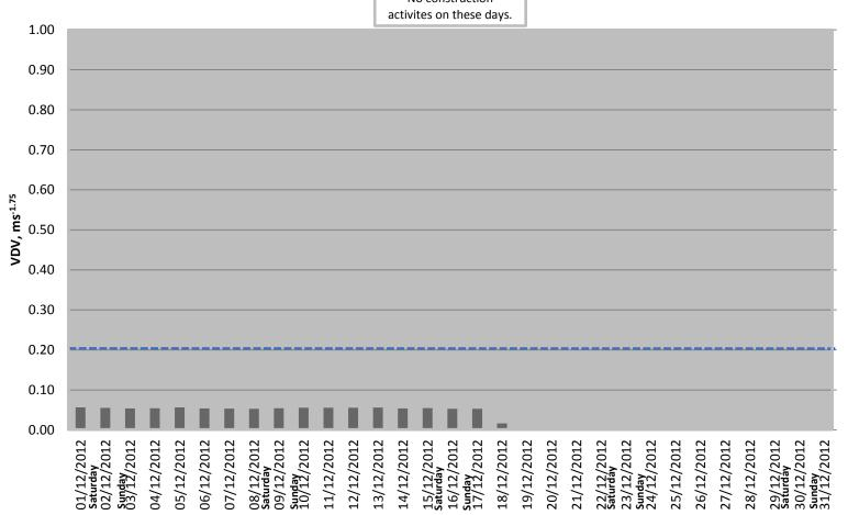
VDV threshold for Education establishments, offices and similar is 0.40ms<sup>-1.75</sup> and Commercial is 0.80ms<sup>-1.75</sup>. Therefore it may be necessary to adjust the threshold displayed
