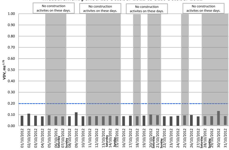
A transfer function equivalent to doubling the night-time VDV measurements has been applied to obtain values representative of an upstairs, mid-floor receptor location. VDV threshold for Education establishments, offices and similar is 0.40ms<sup>-1.75</sup> and Commercial is 0.80ms<sup>-1.75</sup>. Therefore it may be necessary to adjust the threshold displayed on the graph if buildings other than residential dwellings are being assessed.
