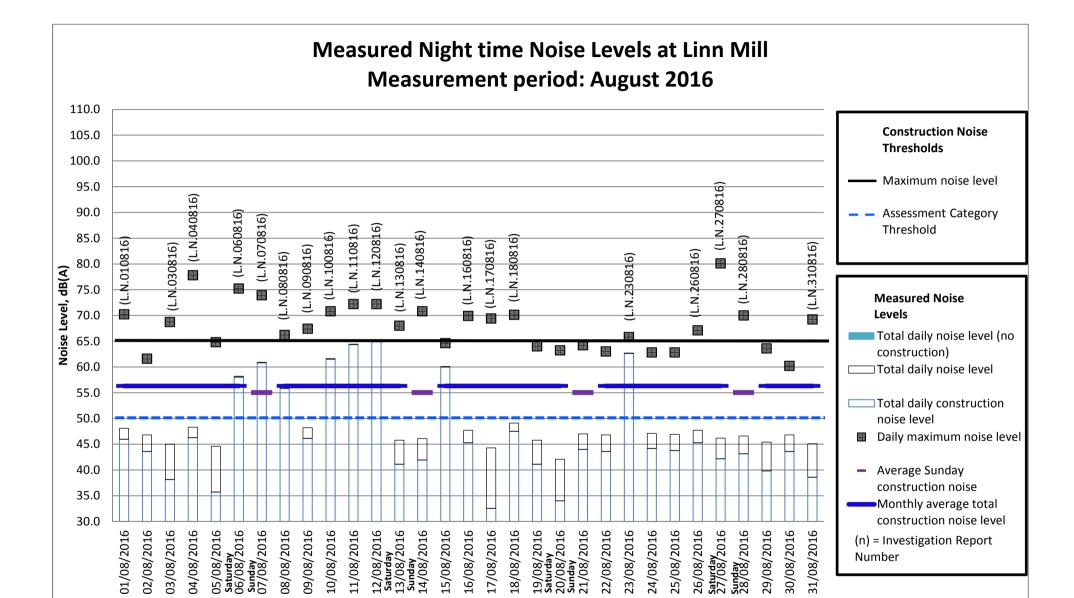
**Note:** After investigation, it was concluded that the exceedance of the LAeq 'Total Daily Construction' on the 10th,11th, 12th and 23rd were caused by a generator being left on in close proximity of the noise monitor (see 2.9 of report). Other exceedances were caused by birds.
