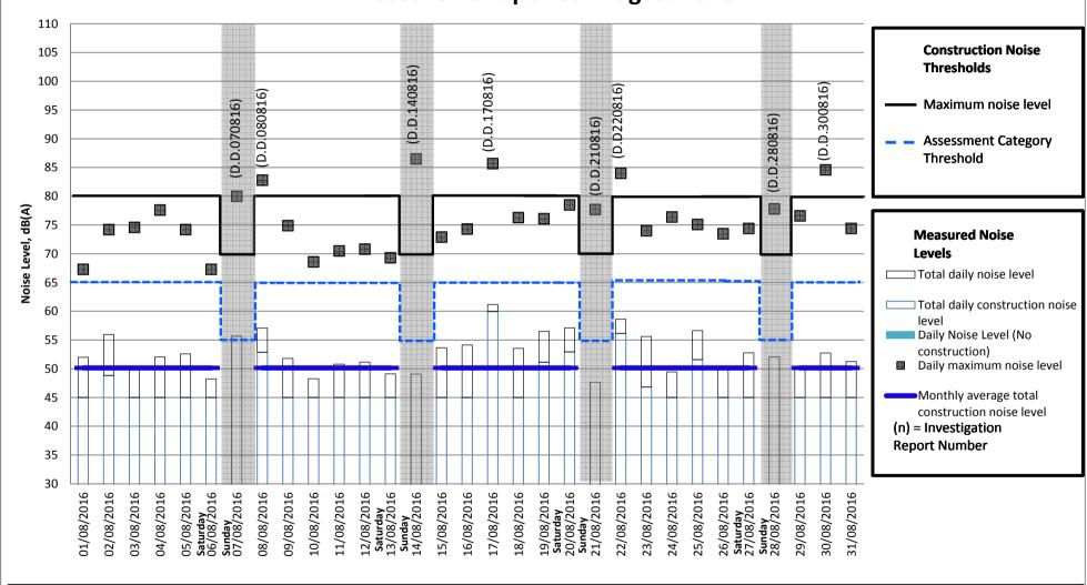
Note: The grey areas of the chart represent days on which no construction works have been conducted;
