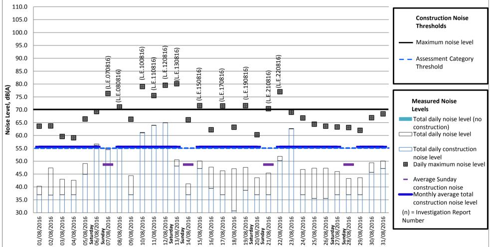
**Note:** After investigation, it was concluded that the exceedance of the LAeq 'Total Daily Construction' on the 10th, 11th, 12th and 23rd were cased by a generator being left on in close proximity of the noise monitor (see 2.9 of report).
