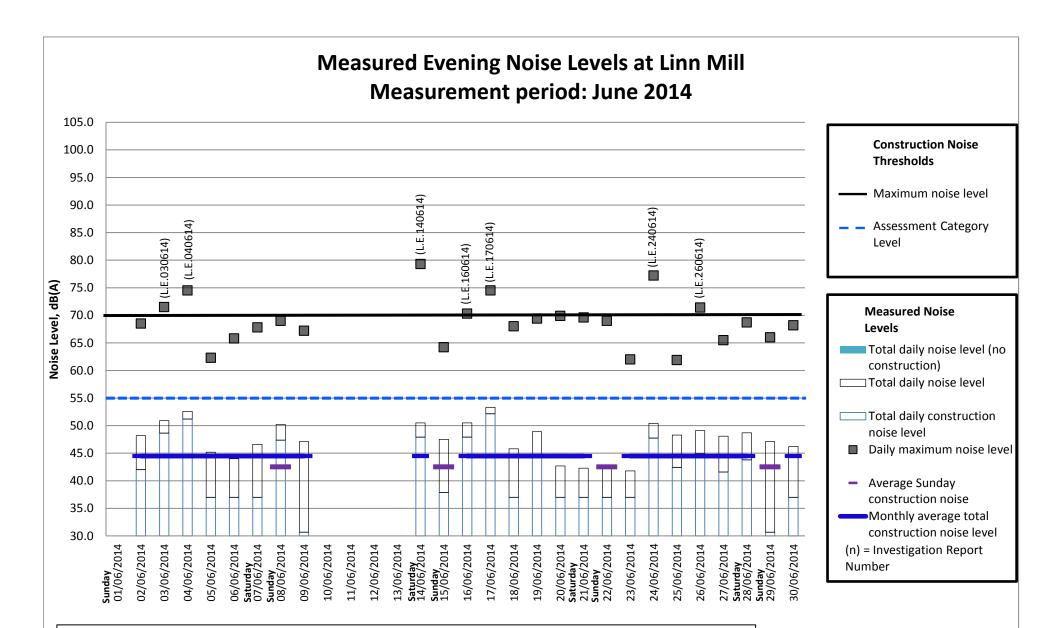
Note: Data is missing from 01/06/14 & 10/06/14 - 13/06/14 due to a device error
