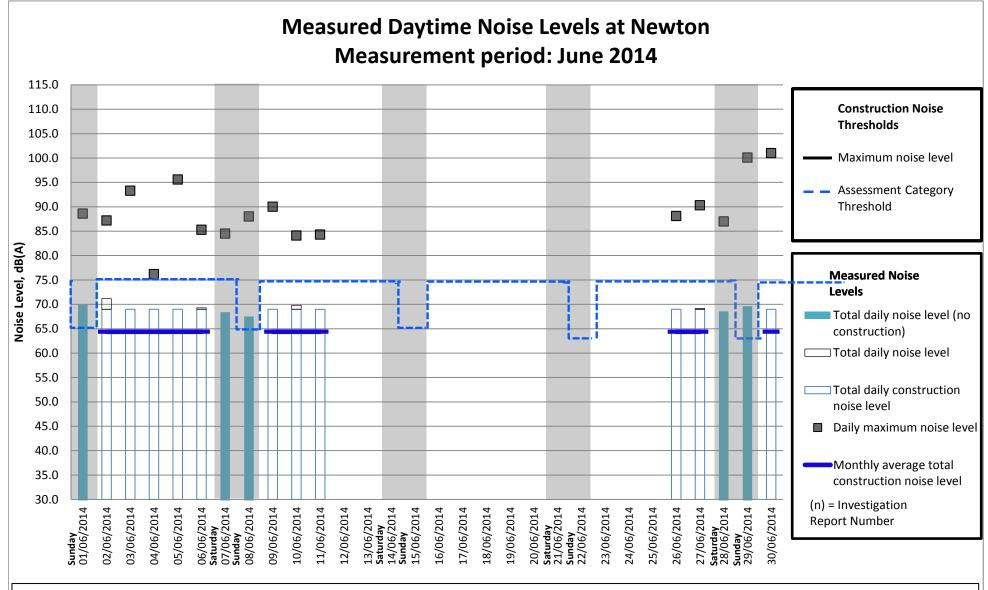
Note: The grey areas of the chart represent days on which no construction works have been conducted. It should be noted that the measured noise levels Mon - Fri can not be attributed to construction works due to the considerable distance (1.75 kilometers) between this monitoring location and the closest construction works. Data is missing from 12/06/14 - 25/06/14 due to device error and inaccessibility to this device.
