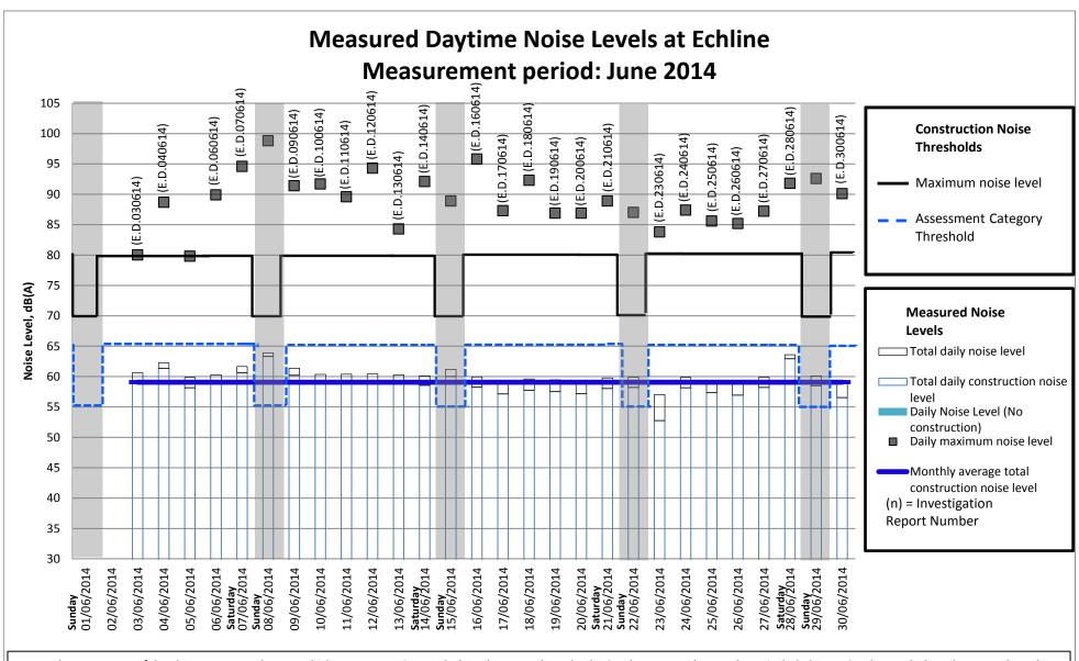
**Note:** The grey areas of the chart represent days on which no construction works have been conducted. The Sunday average has not been included as no Sunday works have been conducted at this location. Data is missing from 01/06/14 & 02/06/14 due to a device error.
