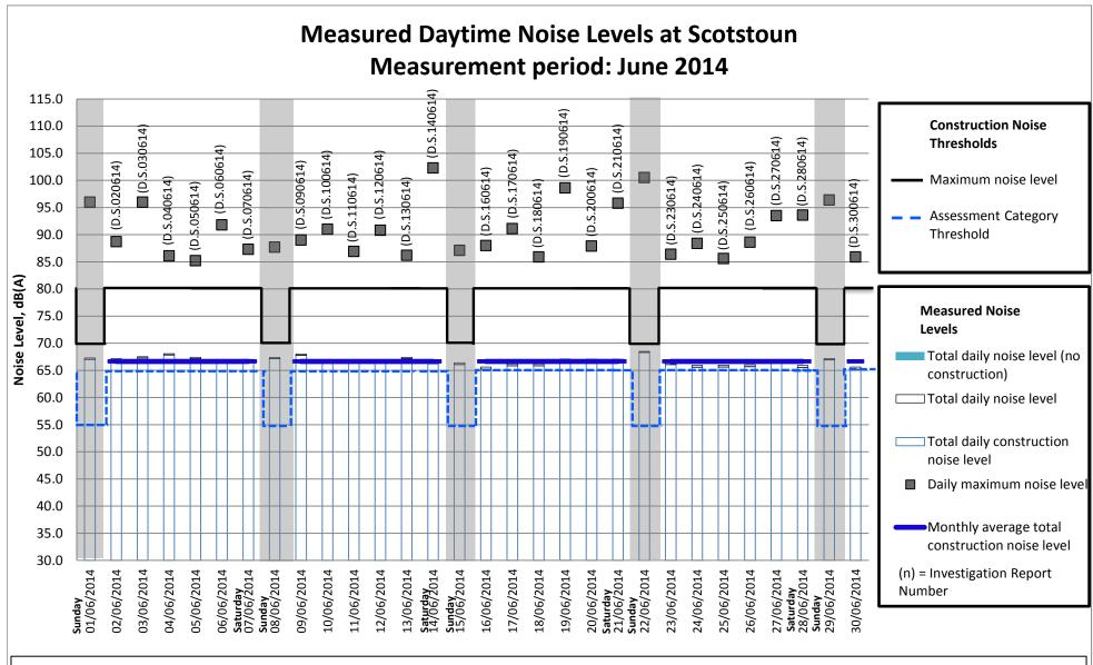
**Note:** The grey areas of the chart represent days on which no construction works have been conducted. The monthly average construction noise for Sunday has not been included as no Sunday works have been conducted at this location.
