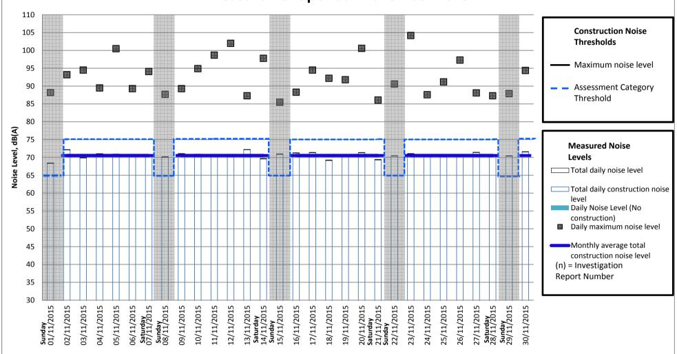
**Note:** The grey areas of the chart represent days on which no construction works have been conducted. It should be noted that the measured noise levels Mon - Fri can not be attributed to construction works due to the considerable distance (1.75 kilometers) between this monitoring location and the closest construction works.
