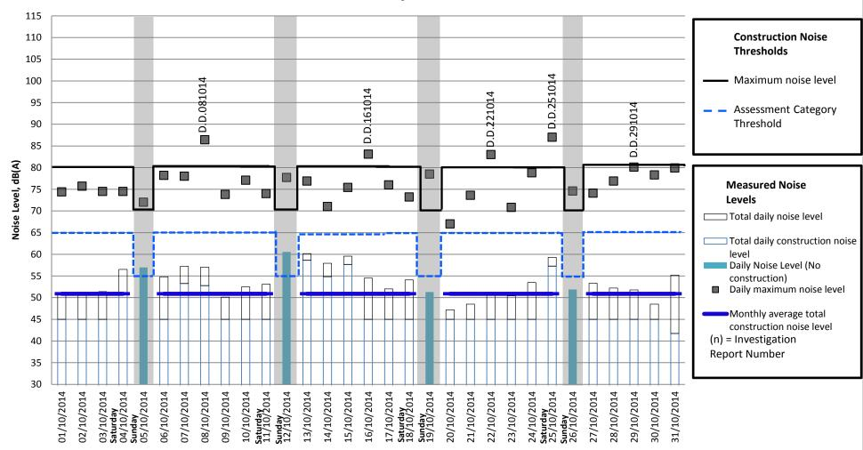
**Note:** The grey areas of the chart represent days on which no construction works have been conducted. The monthly average construction noise for Sunday has not been included as no Sunday works have been conducted at this location.
