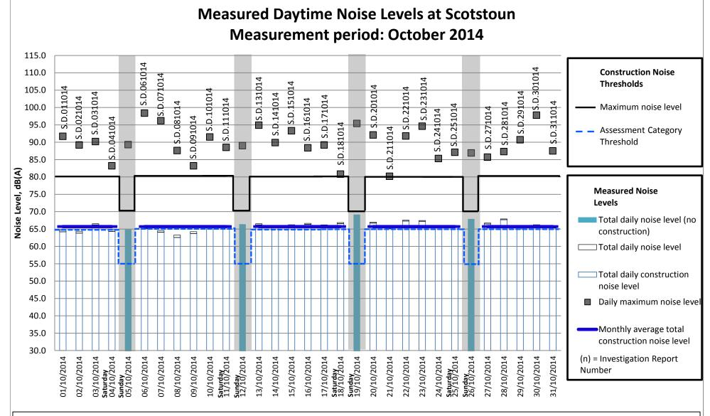
**Note:** The grey areas of the chart represent days on which no construction works have been conducted. The monthly average construction noise for Sunday has not been included as no Sunday works have been conducted at this location .
