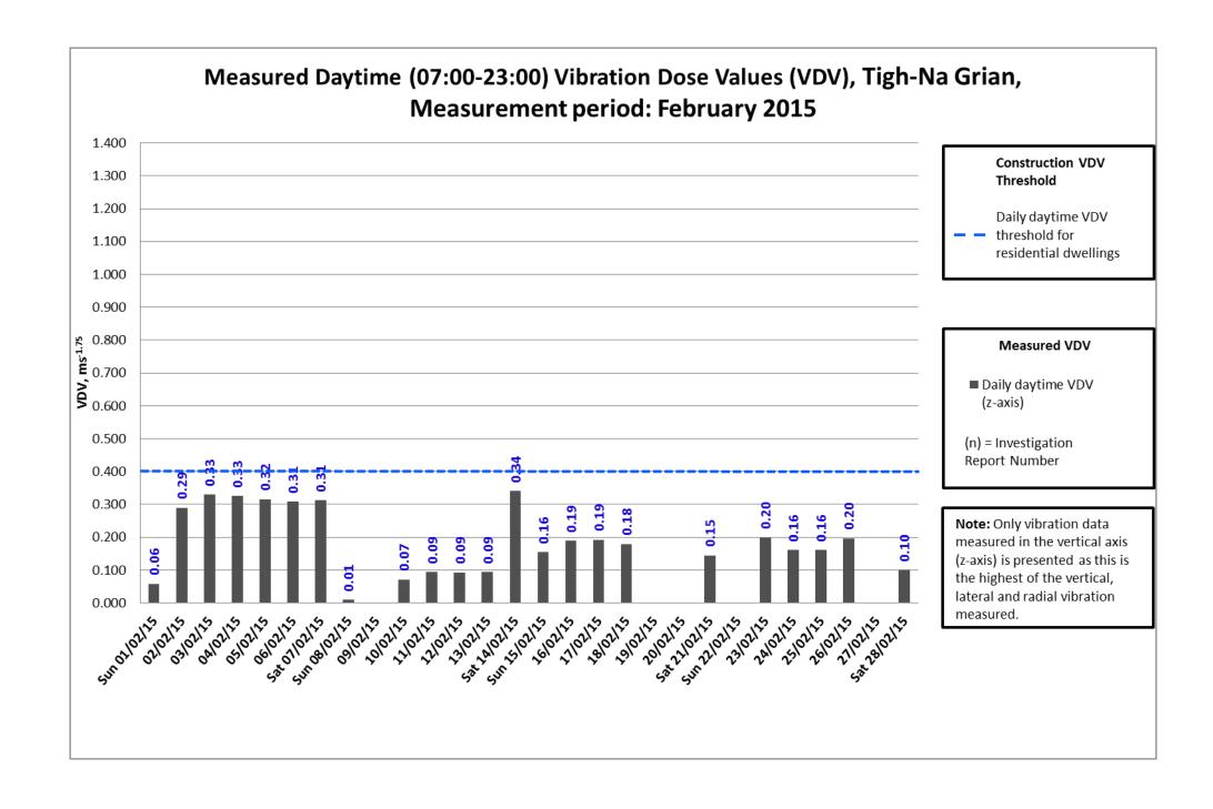
• Data is missing from 09/02/15, 19/02/15, 20/02/15, 22/02/15 and 27/02/15 due to device error.
