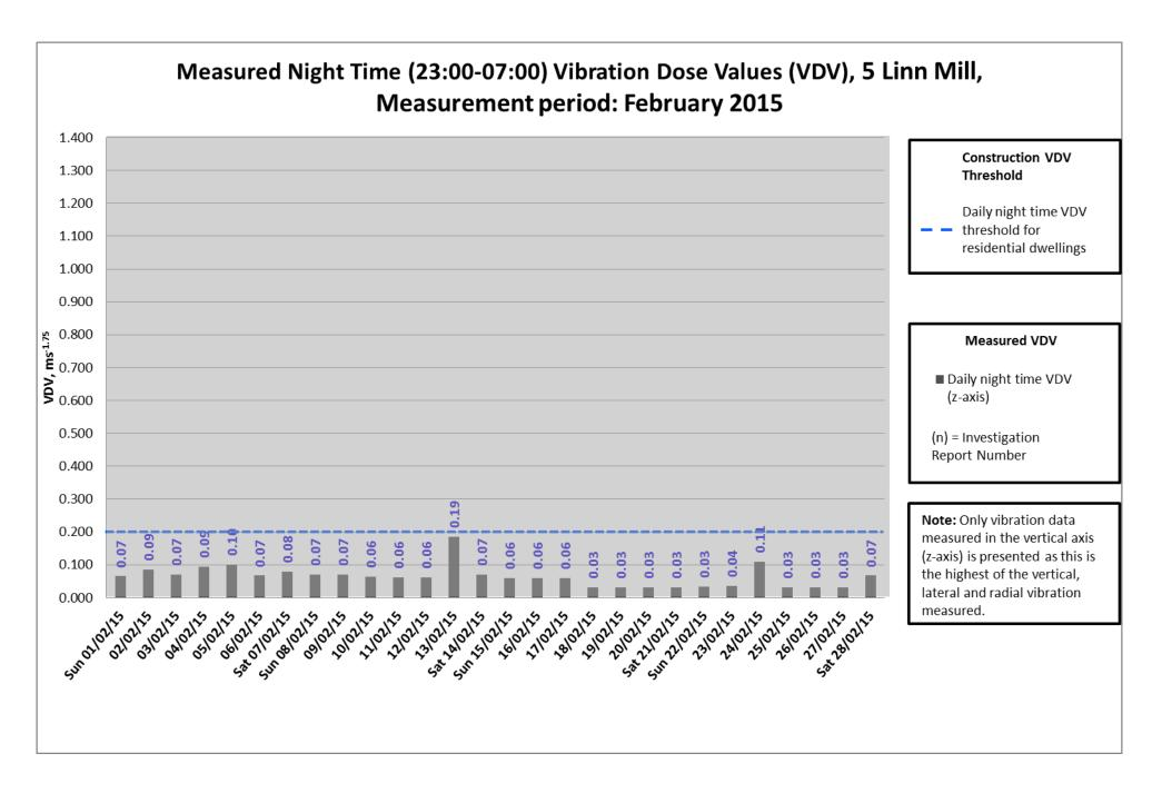
• The grey areas of the chart represent the days on which no construction works were undertaken; no night time works were conducted in the vicinity of the Linn Mill vibration monitor throughout the month of February 2015. This graph is included for illustrative purposes only.
