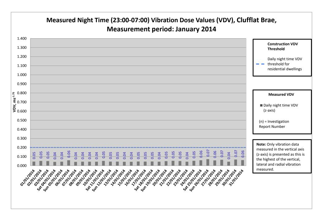
• The grey areas of the chart represent the days on which no construction works were undertaken; no night time works were conducted in the vicinity of the Clufflat Brae vibration monitor throughout the month of January 2014. This graph is included for illustrative purposes only.
