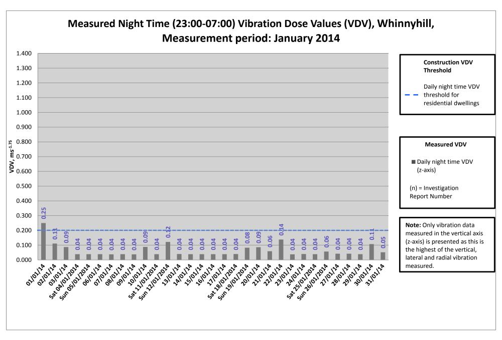
• The grey areas of the chart represent the days on which no construction works were undertaken; no night time works were conducted in the vicinity of the Whinnyhill vibration monitor throughout the month of January 2014. This graph is included for illustrative purposes only.
