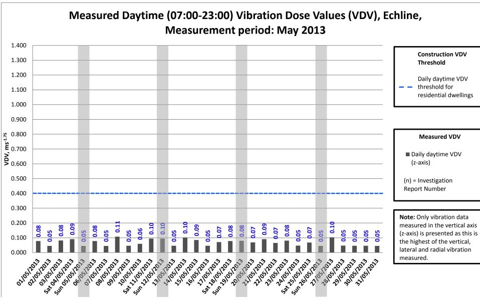
• The grey areas of the chart represent the days on which no construction works were undertaken; no works were conducted on Sundays.
