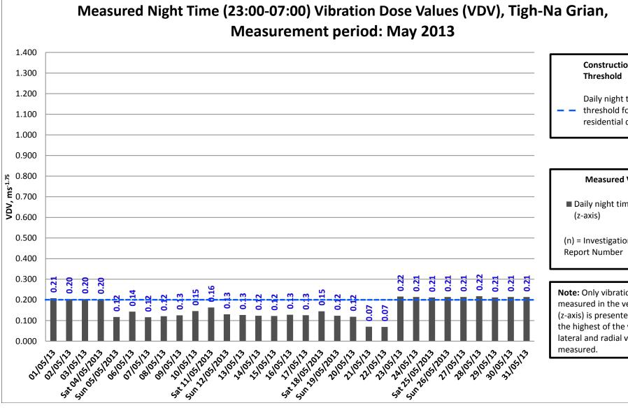
• The VDV exceedances recorded during May 2013 have been investigated, and cannot have been generated as a result of FCBC construction, as the only the works to be conducted throughout the month of May in vicinity of the monitor, was airlifting works at the North Tower, which is over 250m from the monitor, and did not involve the use of any vibration inducing plant or equipment.
