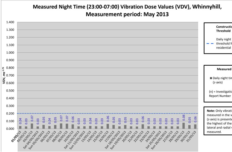
• The grey areas of the chart represent the days on which no construction works were undertaken; no night time works were conducted in the vicinity of the Whinnyhill vibration monitor throughout the month of May 2013. This graph is included for illustrative purposes only.
