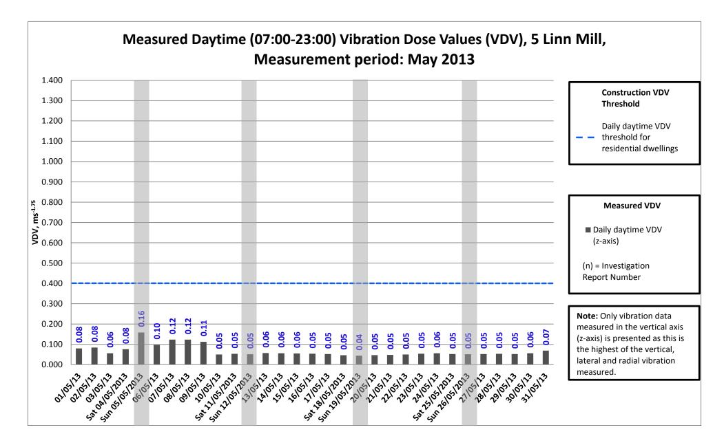
• The grey areas of the chart represent the days on which no construction works were undertaken; no works were conducted on Sundays.
