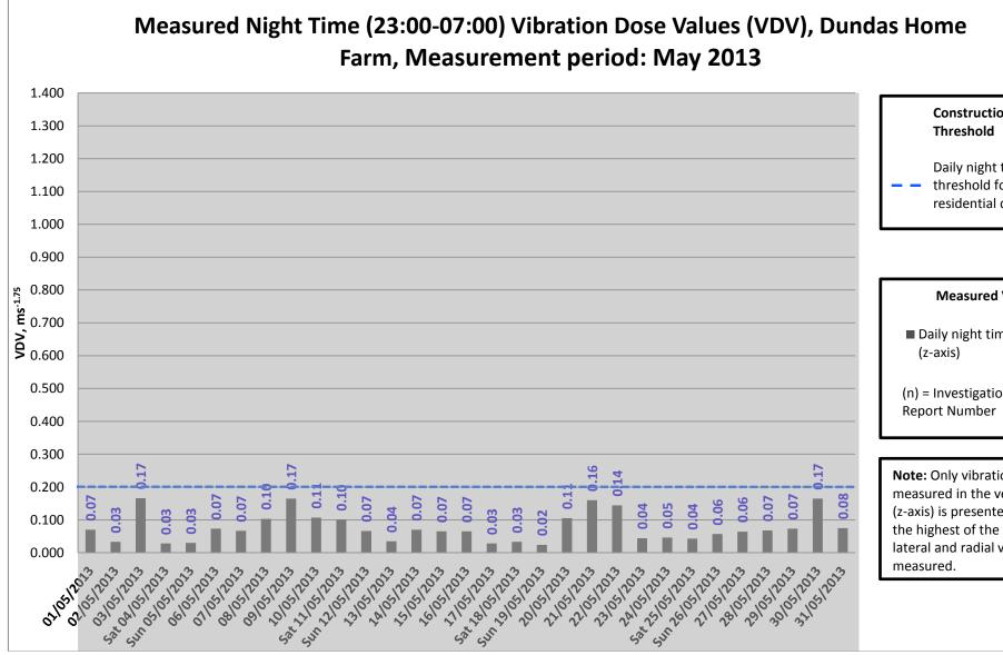
• The grey areas of the chart represent the days on which no construction works were undertaken; no night time works were conducted in the vicinity of the Dundas vibration monitor throughout the month of May 2013. This graph is included for illustrative purposes only.
