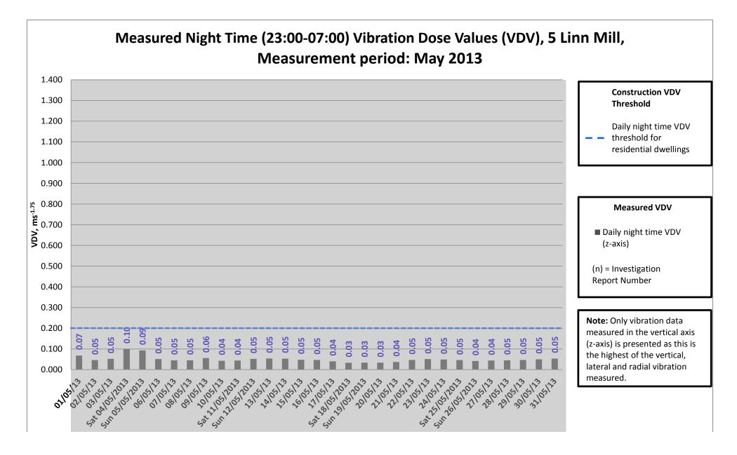
• The grey areas of the chart represent the days on which no construction works were undertaken; no night time works were conducted in the vicinity of the Linn Mill vibration monitor throughout the month of May 2013. This graph is included for illustrative purposes only.
