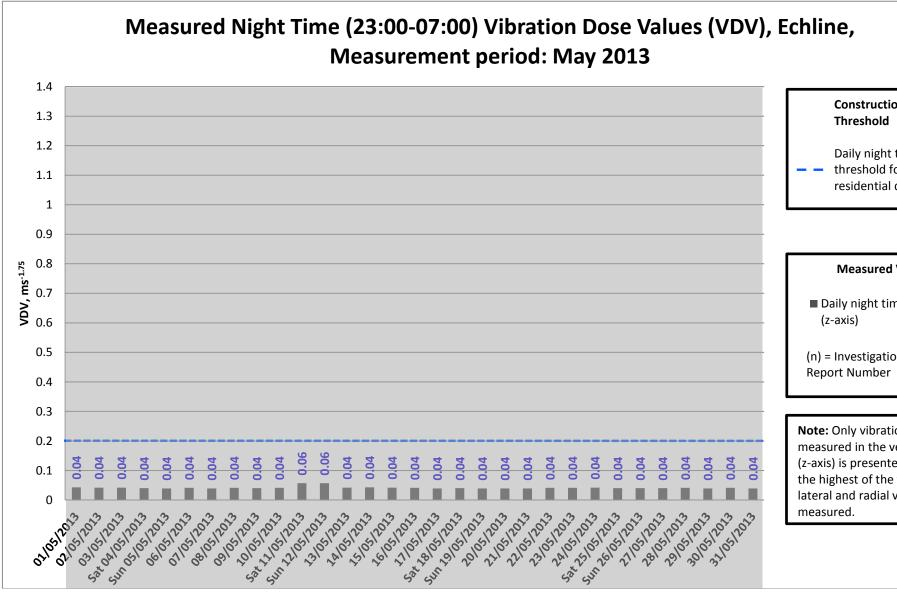
• The grey areas of the chart represent the days on which no construction works were undertaken; no night time works were conducted in the vicinity of the Echline vibration monitor throughout the month of May 2013. This graph is included for illustrative purposes only.
