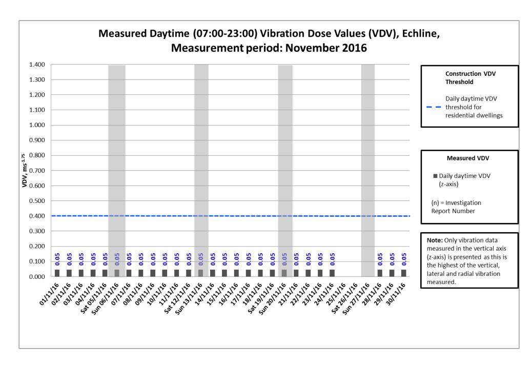
Data missing on the 25<sup>th</sup> - 27<sup>th</sup> November was caused by electrical issue with monitor.
