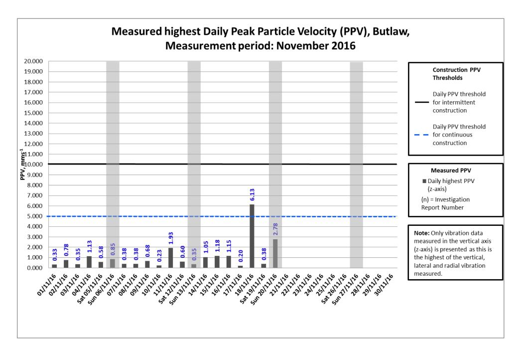
Data missing on the  $21^{st} - 30^{th}$  November was caused by electrical issue with monitor.
