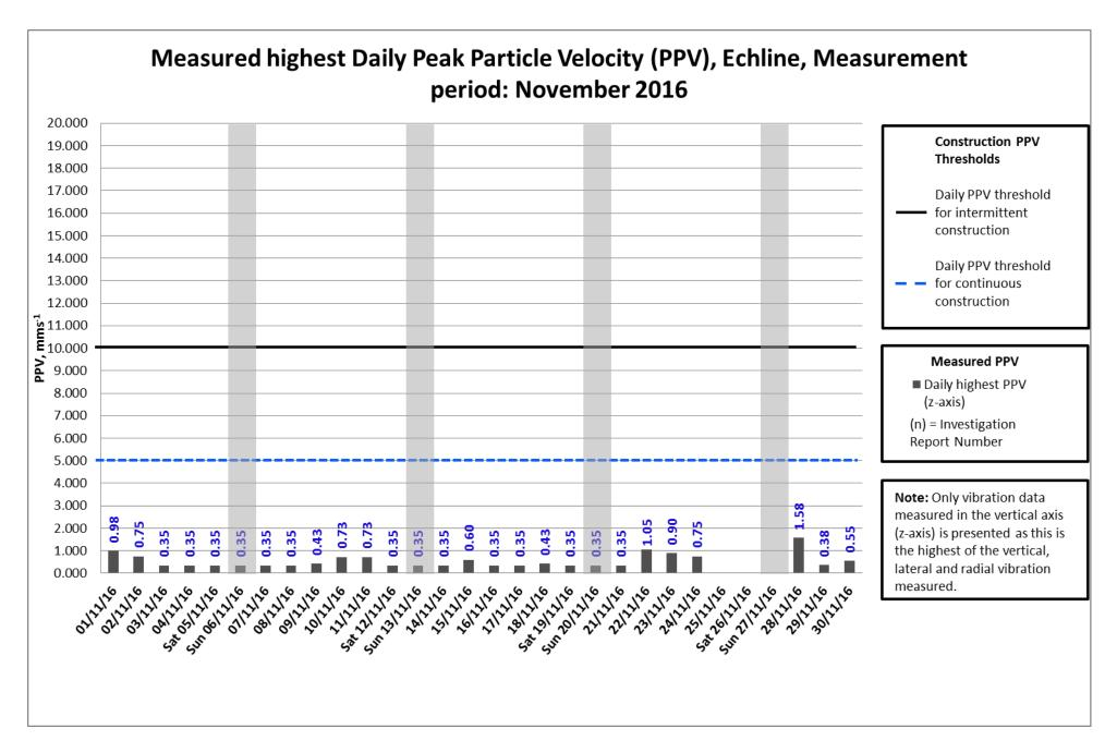
Data missing on the 25<sup>th</sup> - 27<sup>th</sup> November was caused by electrical issue with monitor.
