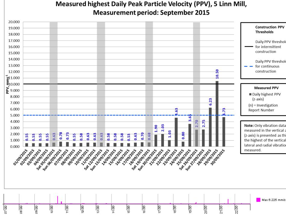
Exceedances on the 28/09/2015 and on the 29/09/2015 have been investigated and found to be isolated events that are unlikely to be caused by construction related activities. It was also noted that the intermittent vibration levels happened within and out with construction working hours (graph above from the 28/09/2015).
