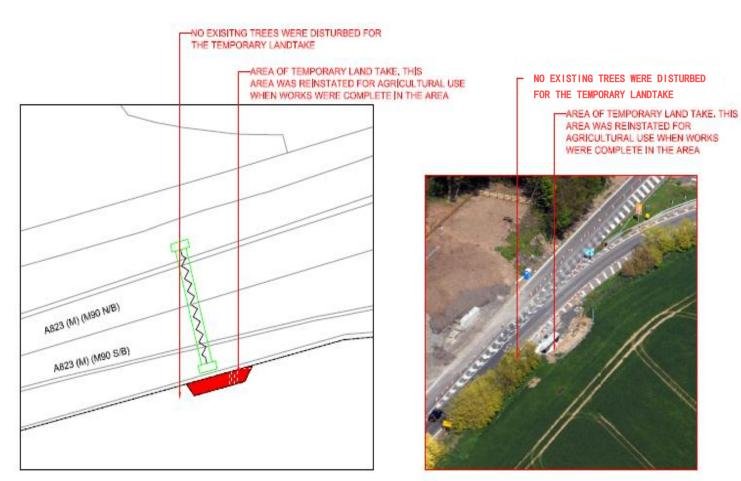
OVERALL SITE VIEW OF G05SB USE OF ADDITIONAL TEMPORARY TRAFFIC MANAGEMENT REDUCED THE AREA OF LAND REQUIRED TO COMPLETE THE WORKS
