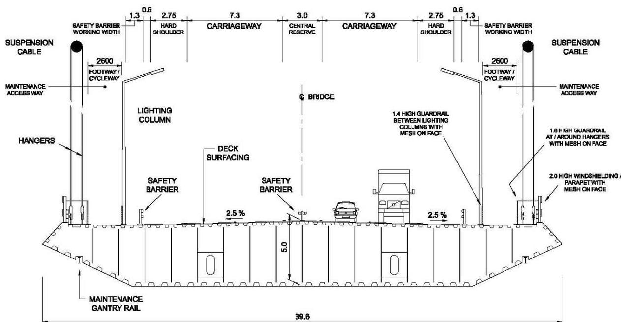
It should be noted that whilst a 2.75 metre wide hardshoulder is appropriate for this design standard it could not support the use of hardshoulder running by public transport modes or HOVs. If this was necessary (and this is described later in Chapters 8 and 9) then the hardshoulder would need to be 3.3 metres wide.
