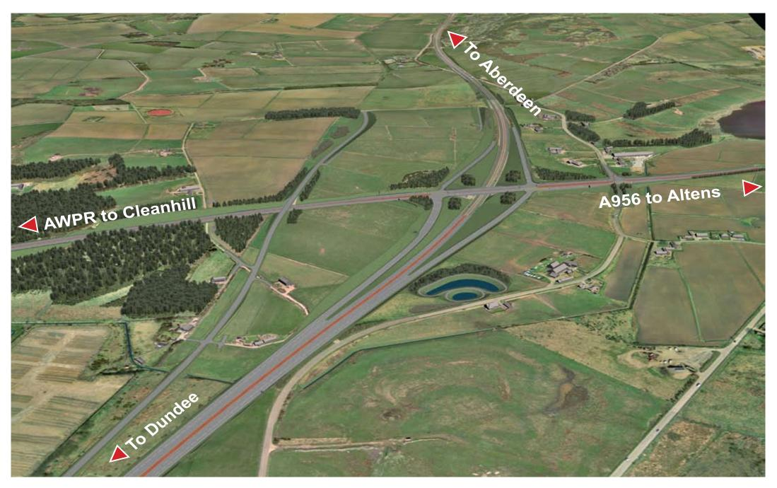
**Charleston Junction (A956)** Signal controlled diamond junction connecting to the A956 and AWPR.
