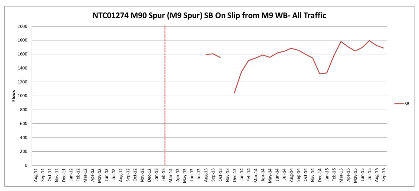
Figure 10 NTC01274 M90 Spur Southbound On Slip from M9 Westbound All Traffic
