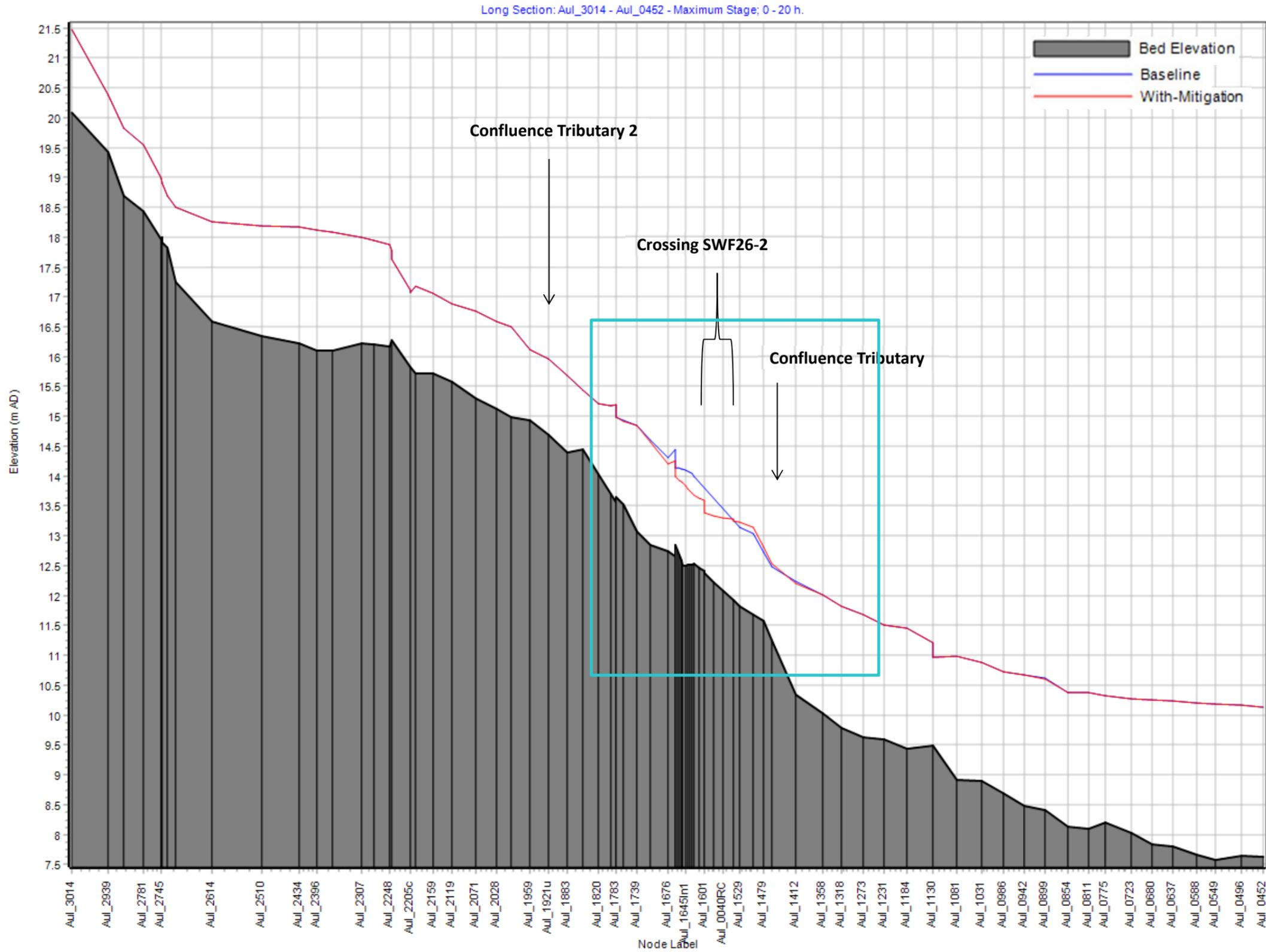
Diagram A2: Auldearn Burn Long Section – 0.5% AEP +CC Event - In-Channel Peak Water Levels - Close up
