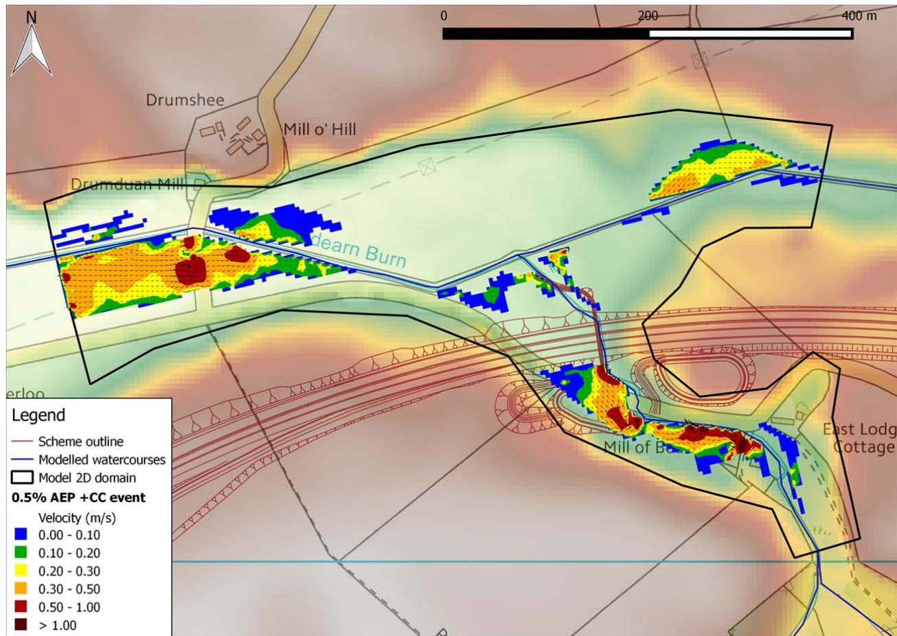
**Diagram 14: 0.5 % AEP +CC Event Maximum Flood Depths – ‘With-Scheme’ Scenario**
