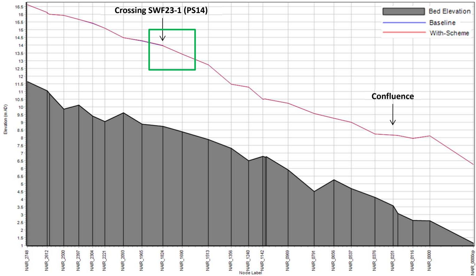
Diagram A2: River Nairn Long Section – 0.5% AEP +CC Event - In-Channel Peak Water Levels - Close up at Scheme Crossing
