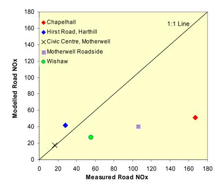
Figure AQ1.2 Measured vs Modelled Nitrogen Dioxide (adjusted)
