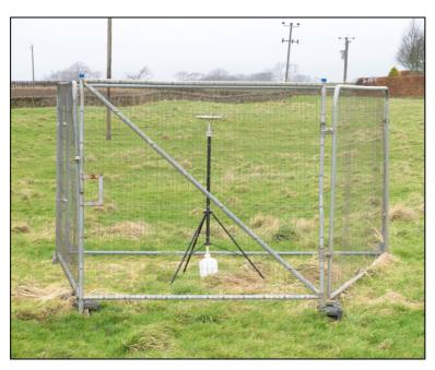
Figure 1: Example of an Installed Frisbee Gauge Meter
