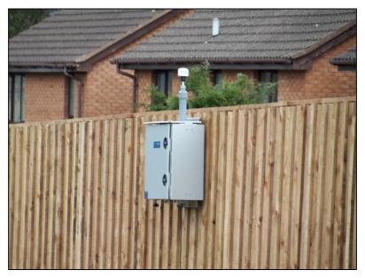
Figure 2: Example of an Automatic Light Scatter Dust Meter
