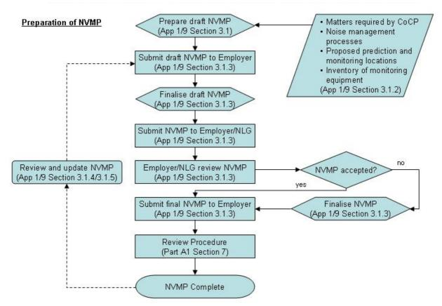
Figure 4.4 Flowchart for the approval and review of the Noise and Vibration Management Plan
