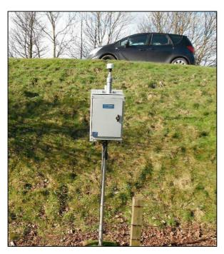
Figure 2: Example of an installed Automatic Light Scatter Dust Meter
