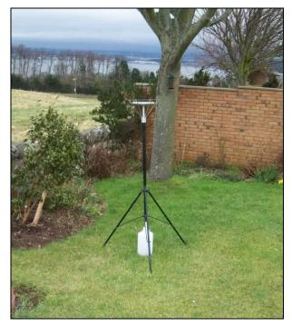
Figure 1: Example of an Installed Frisbee Gauge Meter
