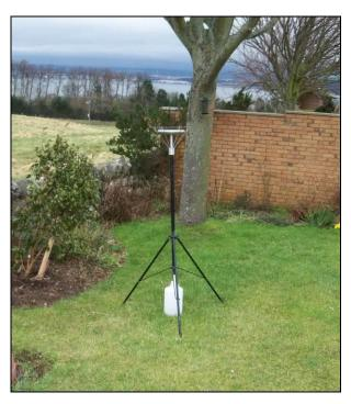
Figure 1: Example of an Installed Frisbee Gauge Meter
