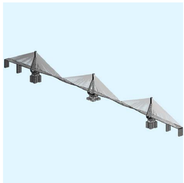
First natural frequency in Torsion
