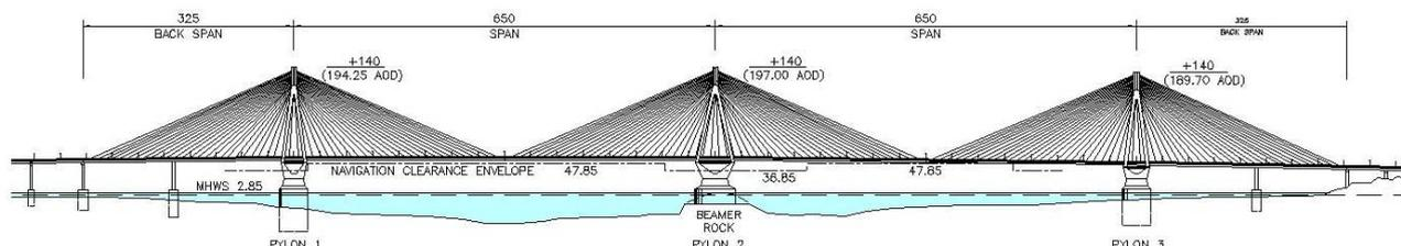
The second type of bridge considered in Corridor D is a cable stayed bridge with two main spans of 650 metres and 40 metre wide deck. This would take around 6 months less to construct than the suspension bridge and its estimated cost is £1.5 billion including network connections and Optimism Bias in Q4 2006 prices.
