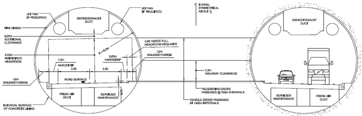
Figure 6.2 – Typical Cross Section for a Mined SCL Tunnel.
