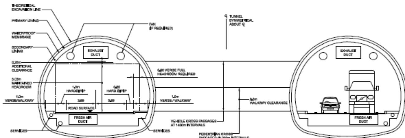
Figure 6.3 – Typical Cross Section for an Immersed Tube Tunnel.
