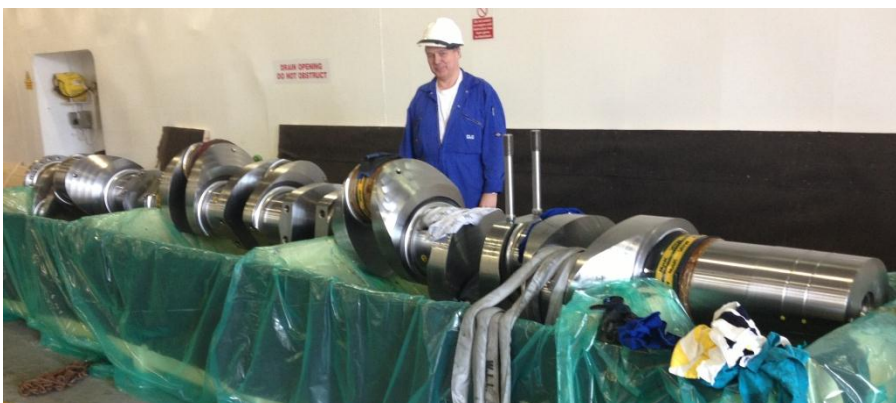
Figure 1. Serco NorthLink Technical Manager, Chris Adams with the replacement crankshaft.
