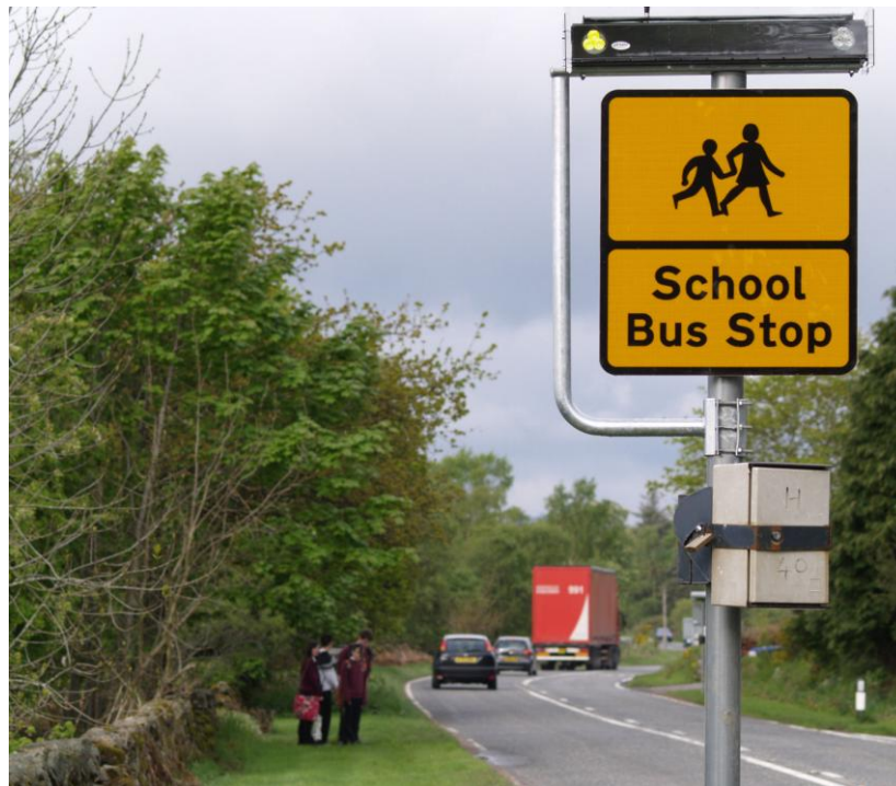
Figure 6-2: SeeMe® school bus stop with flashing lights at the top activated by the presence of pupils carrying transponders
