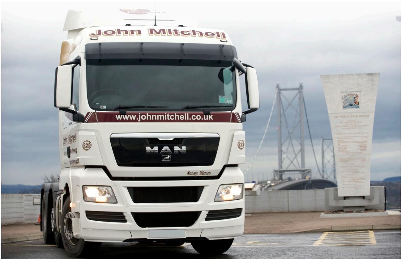
The varied size and shape of the trailers towed by the fleet ensures that good all-round aerodynamic design is required. High roof cabs work well with container and curtain-sided haulage, with trailers up to 14' 6" high. While smaller-cabbed vehicles are specified for use with bulk tanker and local applications, their lower height works well with tankers up to 12' 6" high. All tractor units are specified with full aerodynamic packages at a cost of £750.
