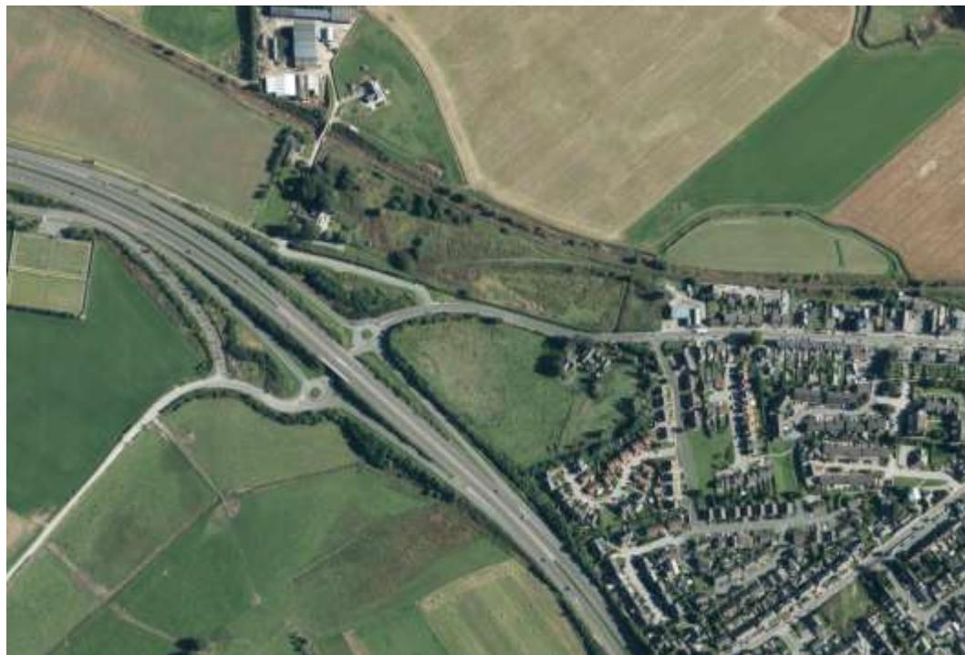
**Figure 4.2.10 Grade separated junction at Kintore**
