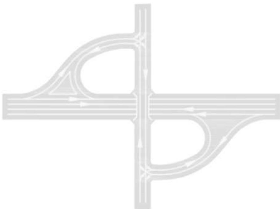
**Figure 4.2.11 Typical Grade Separated Junction Arrangement with Loops**
