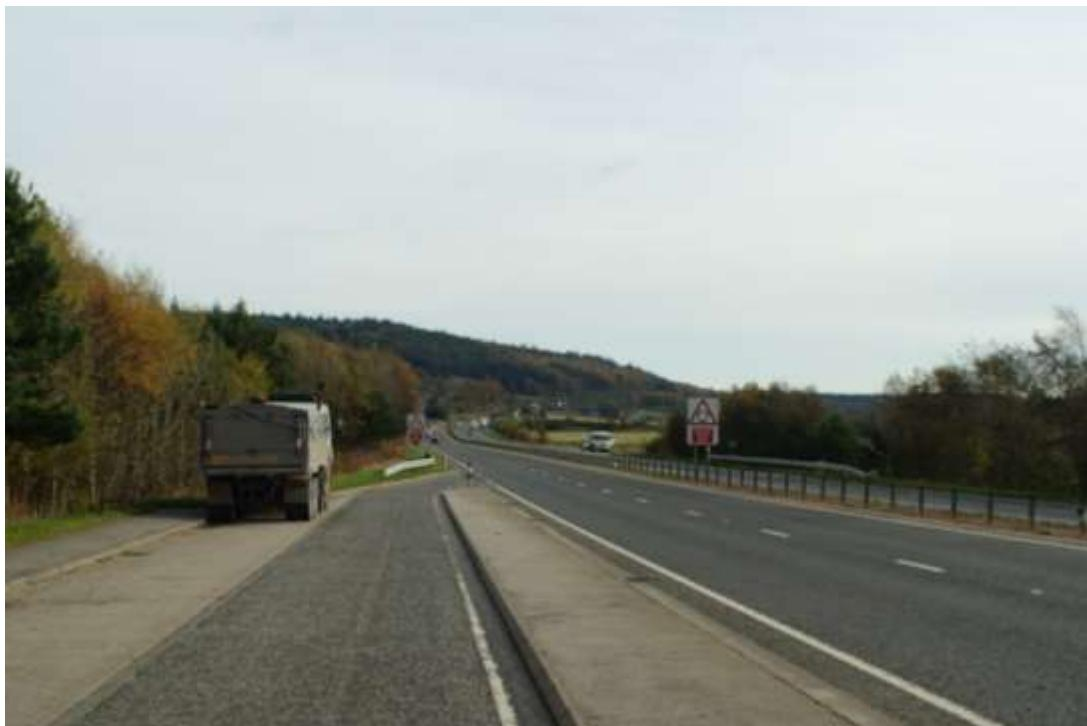
**Figure 4.2.14 Existing Type A Lay-by on dual carriageway section**
