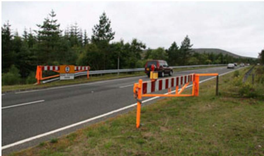
**Figure 8.1 – Snow gates on the A9. These are used to close the road over Drumochter Pass when it is impassable due to snowfall. These and similar installations could also be used to close the road in the event of debris flow.**
