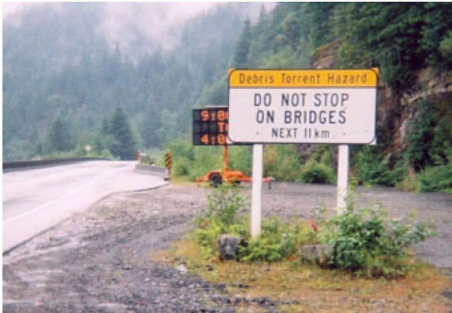
**Figure 8.6 – Sign indicating exposure reduction measures for stream-based debris flow hazards (Vancouver to Whistler, Sea-to-Sky Highway in British Columbia in Canada).**
