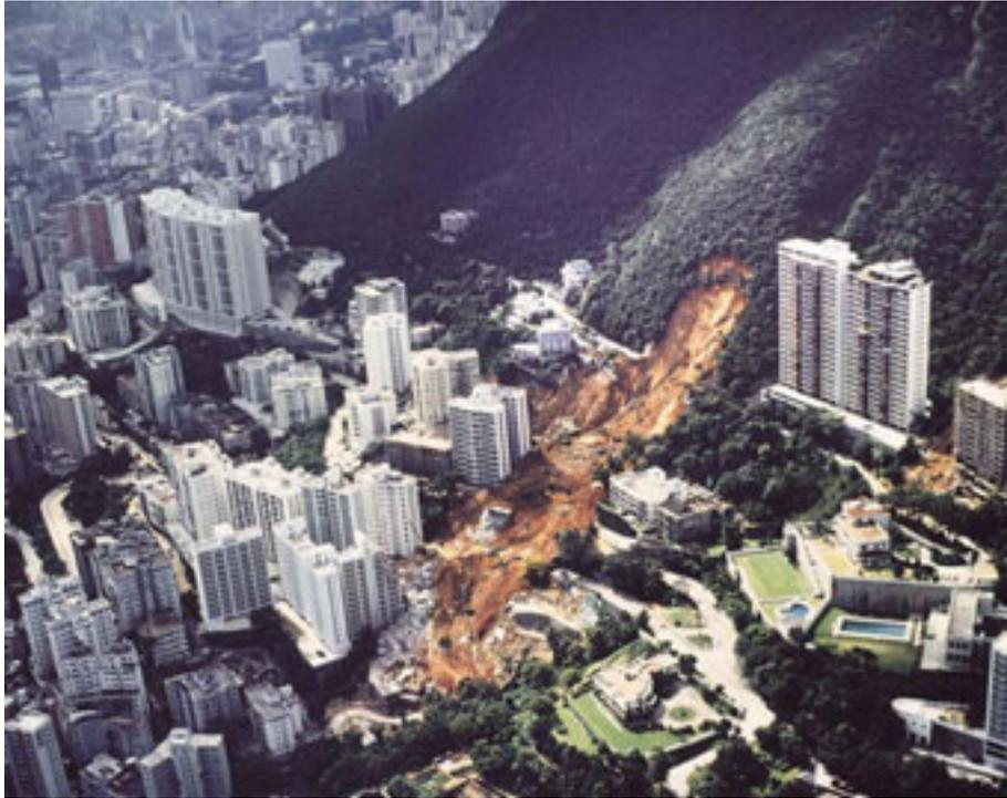
**Figure G.4 – Po Shan Road Landslide, Mid-Levels, Hong Kong Island 18 June 1972. The landslide occurred on a steep hillside above a temporary excavation and demolished a 12-storey building.**
