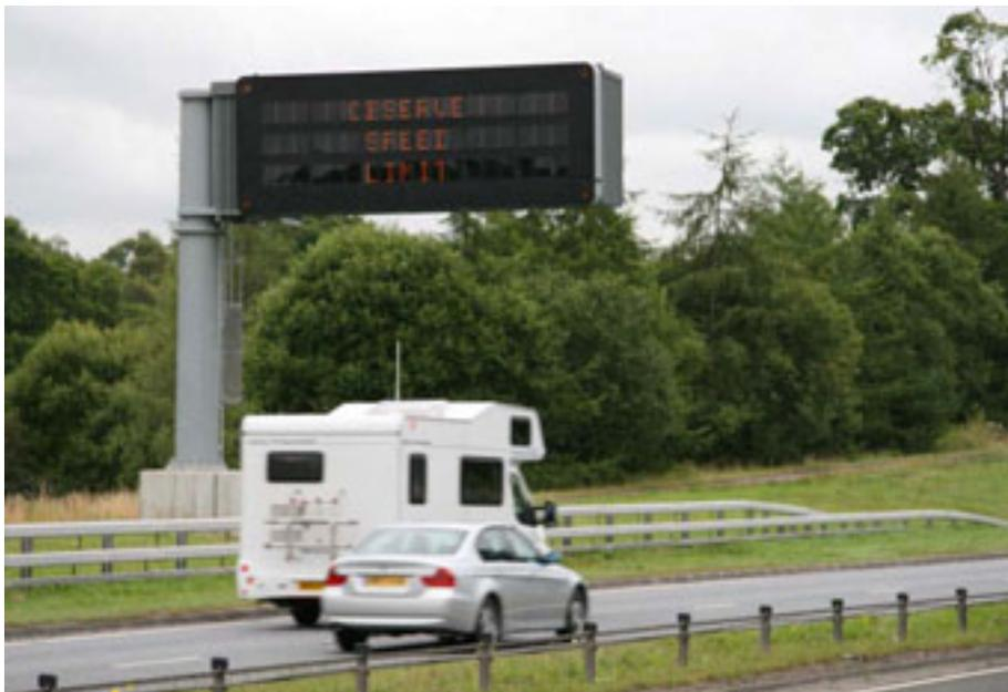
**Figure 8.3 – A variable message sign located on the A9. The network of such signs in Scotland is being significantly increased and will form a crucial part of the strategy for warning road users of hazards including landslides.**
