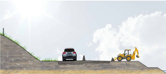
Figure 4.4: Phase 3, traffic moved to new northbound lane
