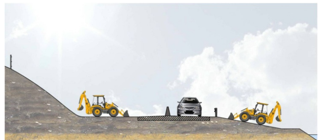
Figure 4.3: Phase 1B, construction of berm on east side
