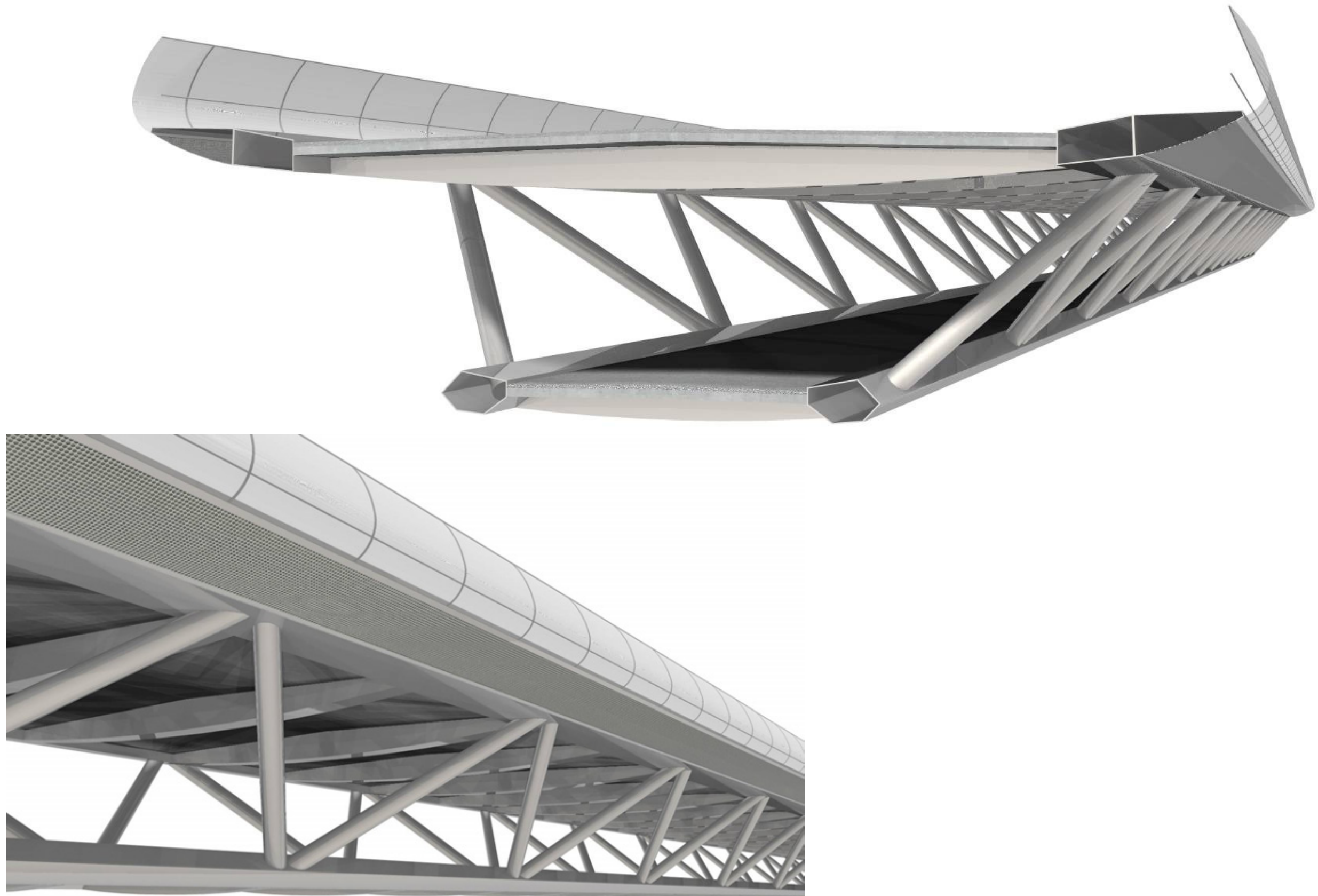
Figure C.24 Two Plane Warren Truss
