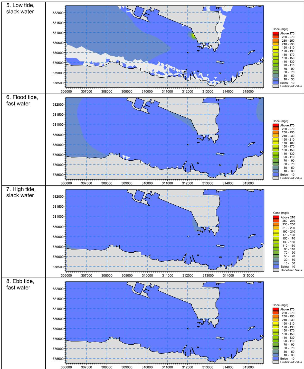
4.5.39 In addition, nine monitoring points are also chosen to record the time series concentration levels in these locations. The nine monitoring points are arranged in a star pattern, with two bursts at 50m and 150m respectively from the centre of each of the construction activity:
