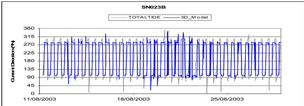
**Diagram 34: SN023D Current- Data vs Model Prediction**
