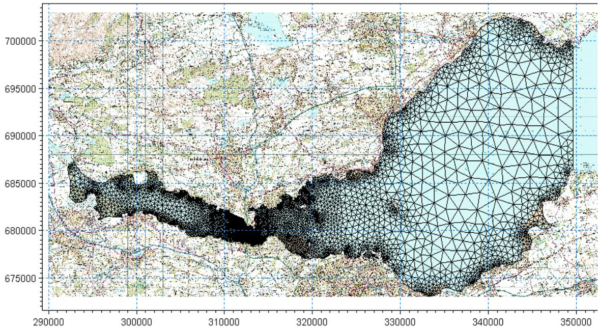
4.3.6 The hydrodynamic model has been calibrated and validated (see Section 1.2) against a range of recorded data obtained from several recognised sources and predicted tidal results produced by the UKHO TOTALTIDE model.
