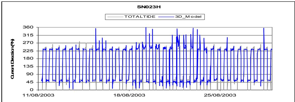
**Diagram 43: SN023I Current – Data vs. Model Prediction**
