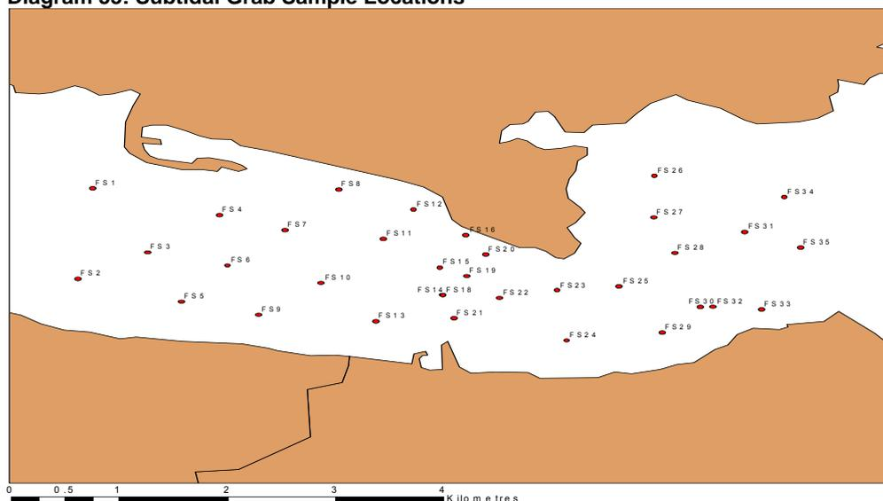
3.4.13 However, these grab samples were taken for the purposes of ecological assessment. Grab sampling is not an ideal method for determining sediment particle size distributions and material classification/fraction (such as clay, silt, sand and gravel) for the purposes of interpretation of sediment transport.
