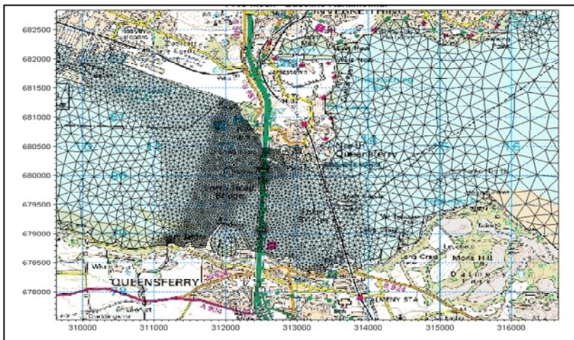
**Diagram 6: Coastal Model Mesh – Eastern Section**
