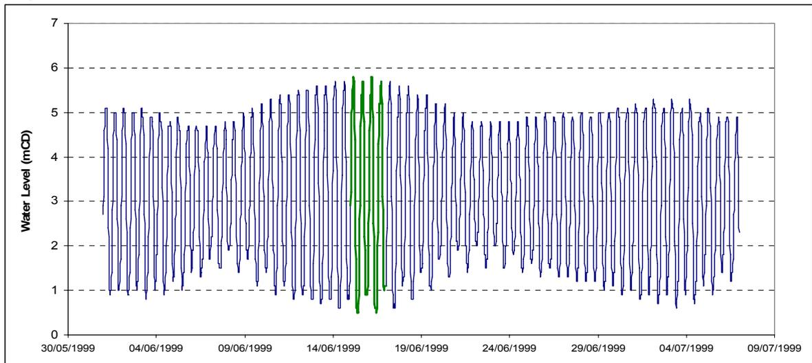
3.2.8 On the eastern boundary of the model, the water level time series at Fidra is used as the boundary condition, as shown in Diagram 47.
