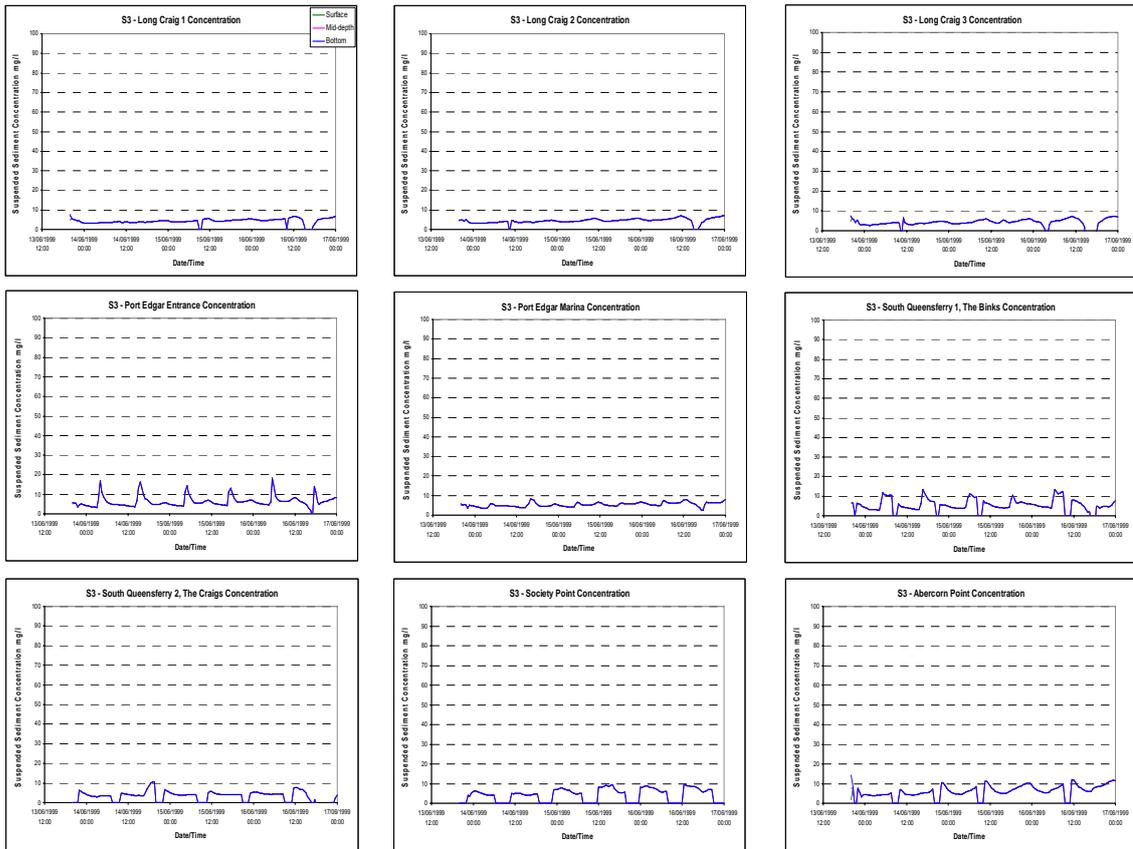
**Diagram 80: Suspended Sediment Concentrations under Scenario ST at Spring Tide (Piling at ST, Bottom Release Only)**
