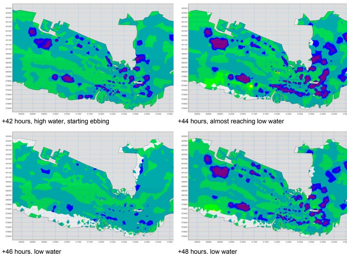
3.4.26 Compared to the baseline condition, the snapshots in the permanent works conditions show widespread increases in bottom speeds in the main channel area but the numerical value is small, in the order of 0.05m/s. After the deduction of the recommended background noise of 0.05m/s, this is reverted to no change at all.
