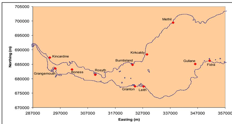
**Diagram 17: Available Current Velocity Measurement/Prediction Points**
