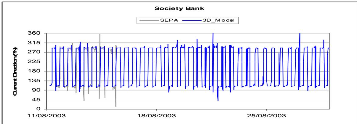
**Diagram 26: SN023F Current – Data vs Model Prediction**
