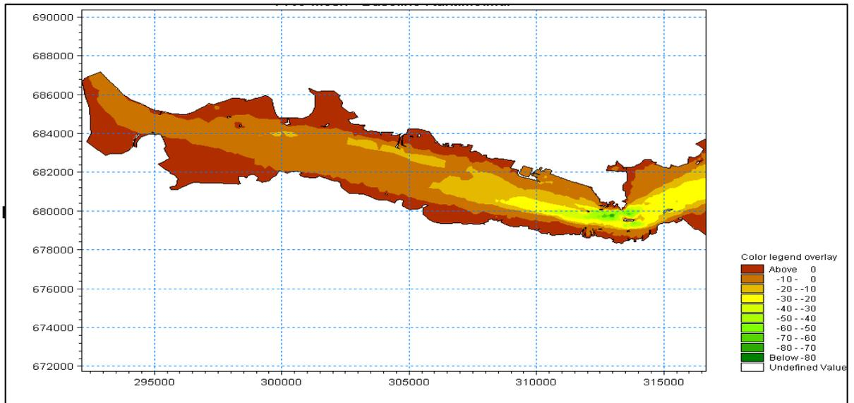
**Diagram 10: The Proposed Scheme Coastal Model Bathymetry – Central and Eastern Section**
