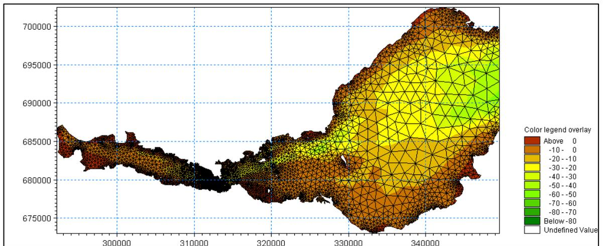
**Diagram 12: The Proposed Scheme Coastal Model Mesh and Bathymetry – Central Section**
