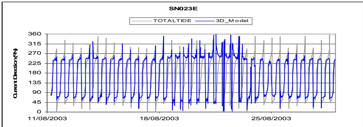
**Diagram 42: SN023H Current – Data vs Model Prediction**
