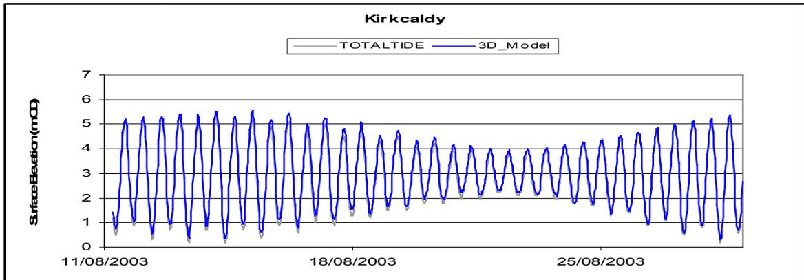
**Diagram 39: Methil Water Level – Data vs Model Prediction**
