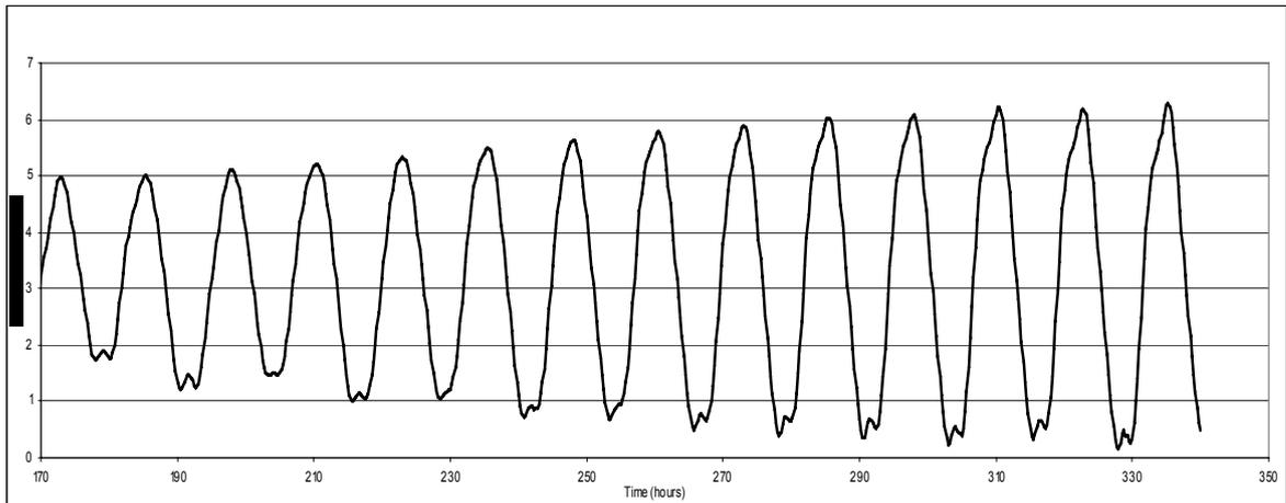
2.4.6 The hydrodynamic model has been able to replicate the lackie tide behaviour in the estuary. Diagram 28 is a shorter plot of the neap tide water levels at Boness (refer to Diagram 23), which is not too far downstream of Kincardine. Even though the plot is for an entirely different time period to Diagram 27, the lackie tide pattern is clearly present.
