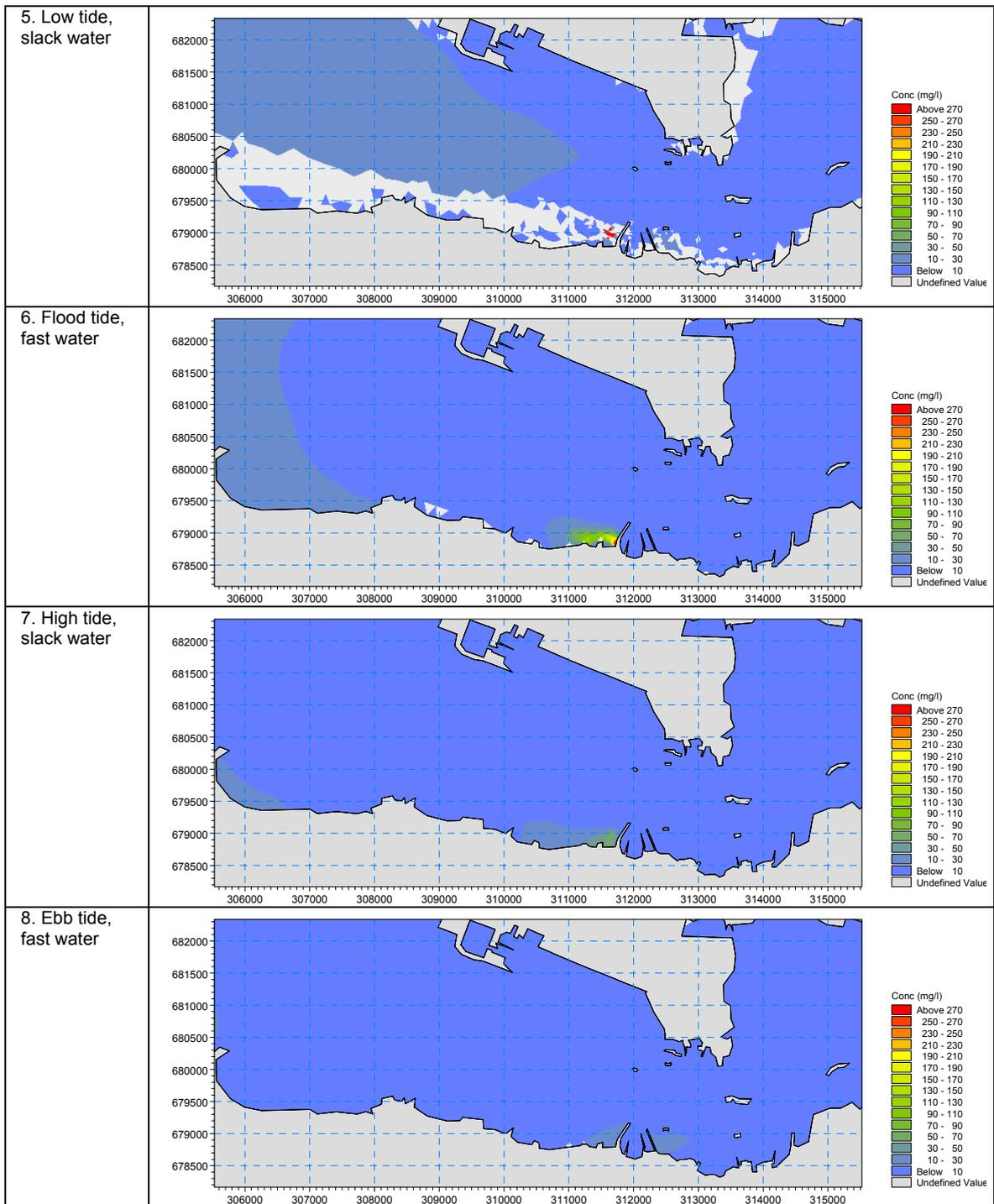
**Diagram 74: Suspended Sediment Concentration Levels at Water Surface for Scenarios ST & N1 at Spring Tide (Piling at ST, Bottom Release Only; Pier N1 Dredging, both Bottom Release and Surface Overspill)**
