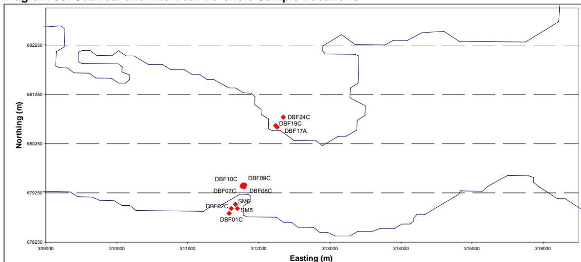
3.4.15 The samples taken consist of sediments found on the seabed penetrating to 1m depth. Given the method of sampling, it is not possible to confirm if the samples are entirely representative of the seabed, however it is possible to determine the general material fractions making up the top 1m layer and this appears to consist of predominantly silts and sands as shown in Table 3.1. The subtidal boreholes are highlighted in yellow.
