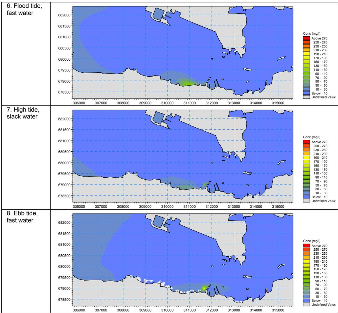
**Diagram 86: Suspended Sediment Concentration Levels at Water Surface for Scenarios ST & N1 at Neap Tide (Piling at ST, Bottom Release Only; Pier N1 Dredging, both Bottom Release and Surface Overspill)**
