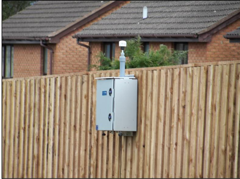
**Figure 2: Example of an Automatic Light Scatter Dust Meter**
