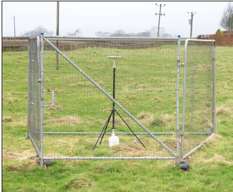
**Figure 1: Example of an Installed Frisbee Gauge Meter**
