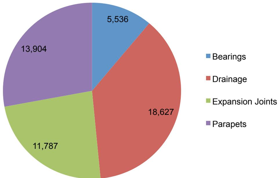
10-Year Work Plan for Structures Maintenance (area treated, m<sup>2</sup>)
