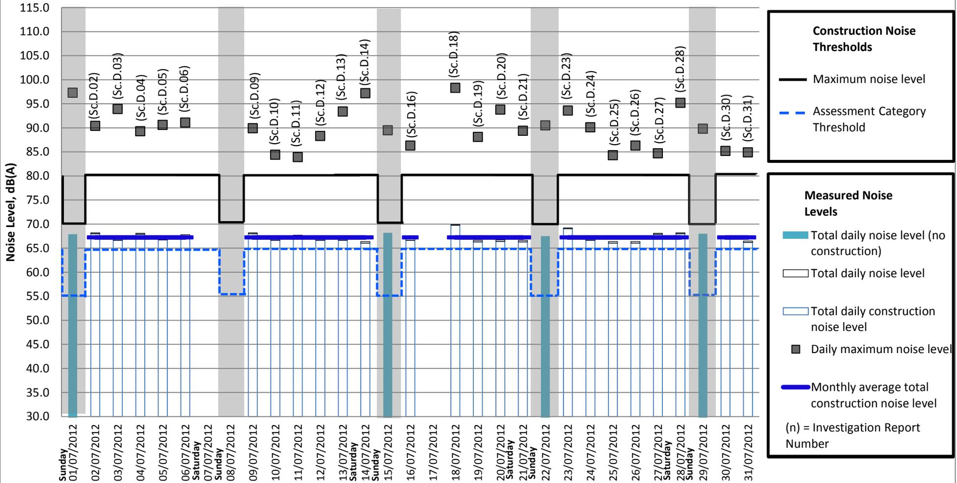
**Note:** The grey areas of the chart represent days on which no construction works have been conducted. The monthly average construction noise for Sunday has not been included as no Sunday works have been conducted at this location. Due to device error, data is missing for 07/07/12, 08/07/12 and 17/07/12.
