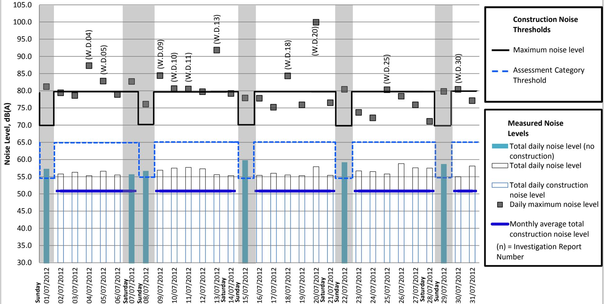
**Note:** The grey areas of the chart represent days on which no construction works have been conducted. The monthly average construction noise for Sunday has not been included as no Sunday works have been conducted at this location .
