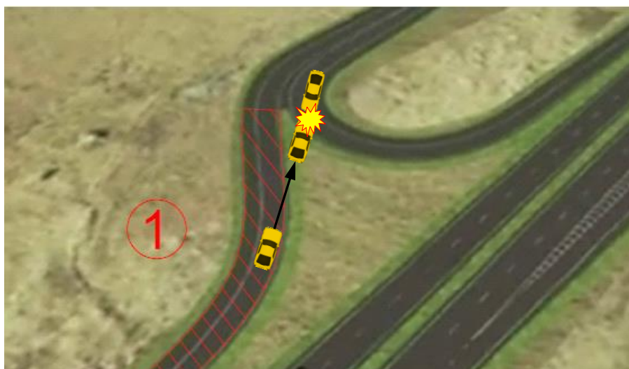
Figure 3 – A Potential Result of a Lack of Median Barrier around the Diverge Areas of Two-Way Slip Roads
