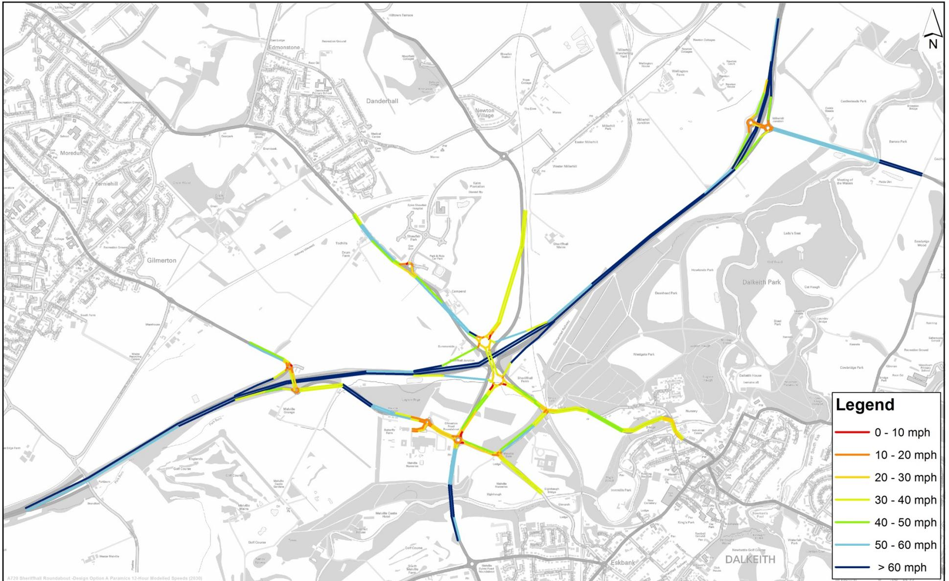
A720 Sheriffhall Roundabout - Design Option A & Paramics 12-Hour Modified Speeds (2030)
