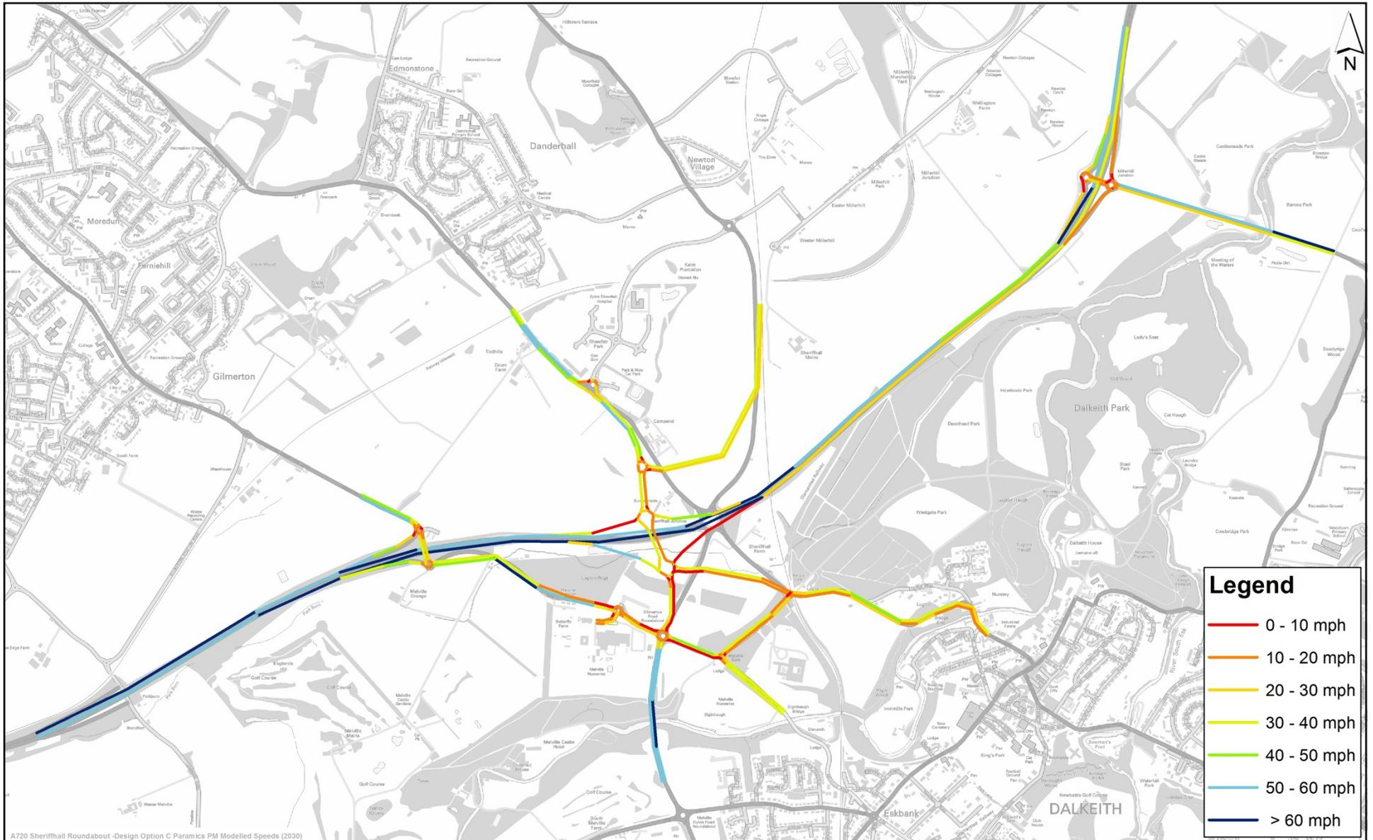
A720 Sheriffhall Roundabout - Design Option C Paramics PM Modelled Speeds (2030)
