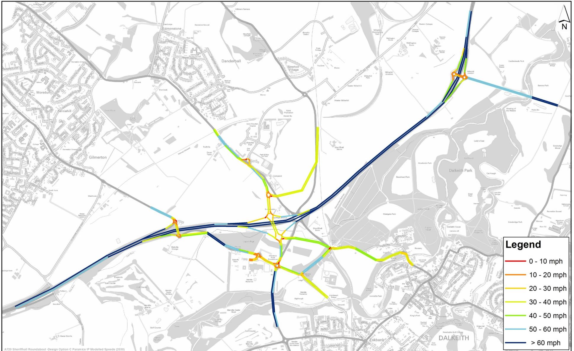
A720 Sheriffhall Roundabout - Design Option C Paramics IP Modelled Speeds (2030)
