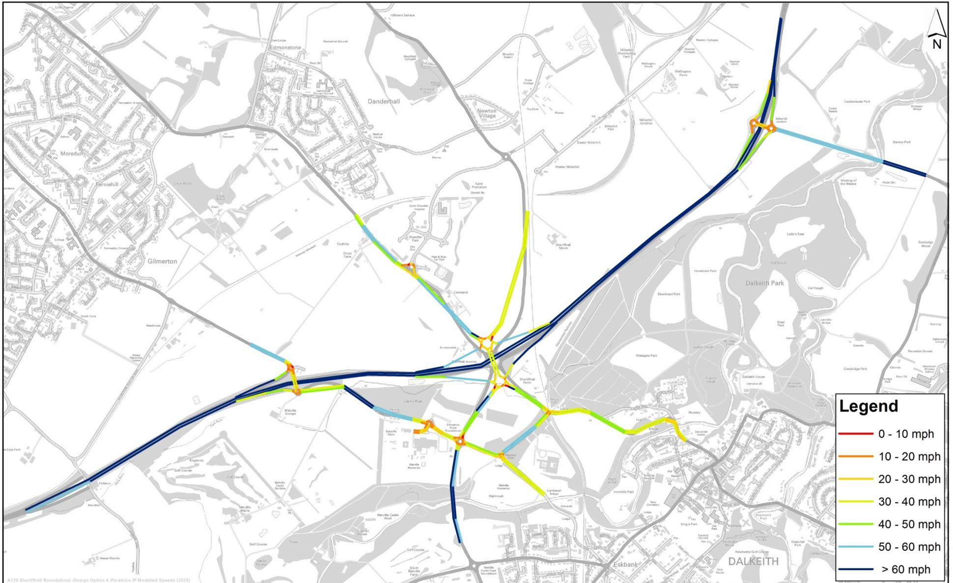
A720 Sheriffhall Roundabout - Design Option A - Paramix of Modelled Speeds (2024)
