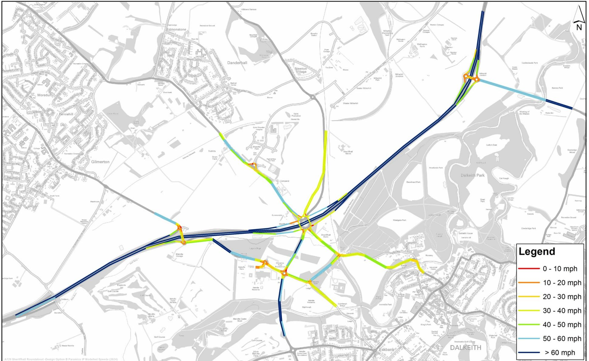
A720 Sheriffhall Roundabout - Design Option B - Paravix (P) Modelled Speeds (2024)
