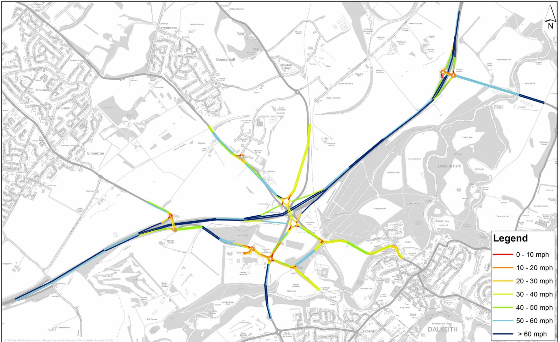
A720 Sheriffhall Roundabout - Design Option A Paramics PM Modelled Speeds (2030)
