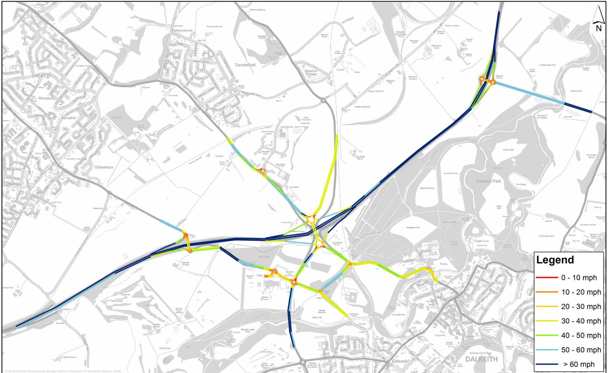
A720 Sheriffhall Roundabout - Design Option A Paramix of Modelled Speeds (2030)
