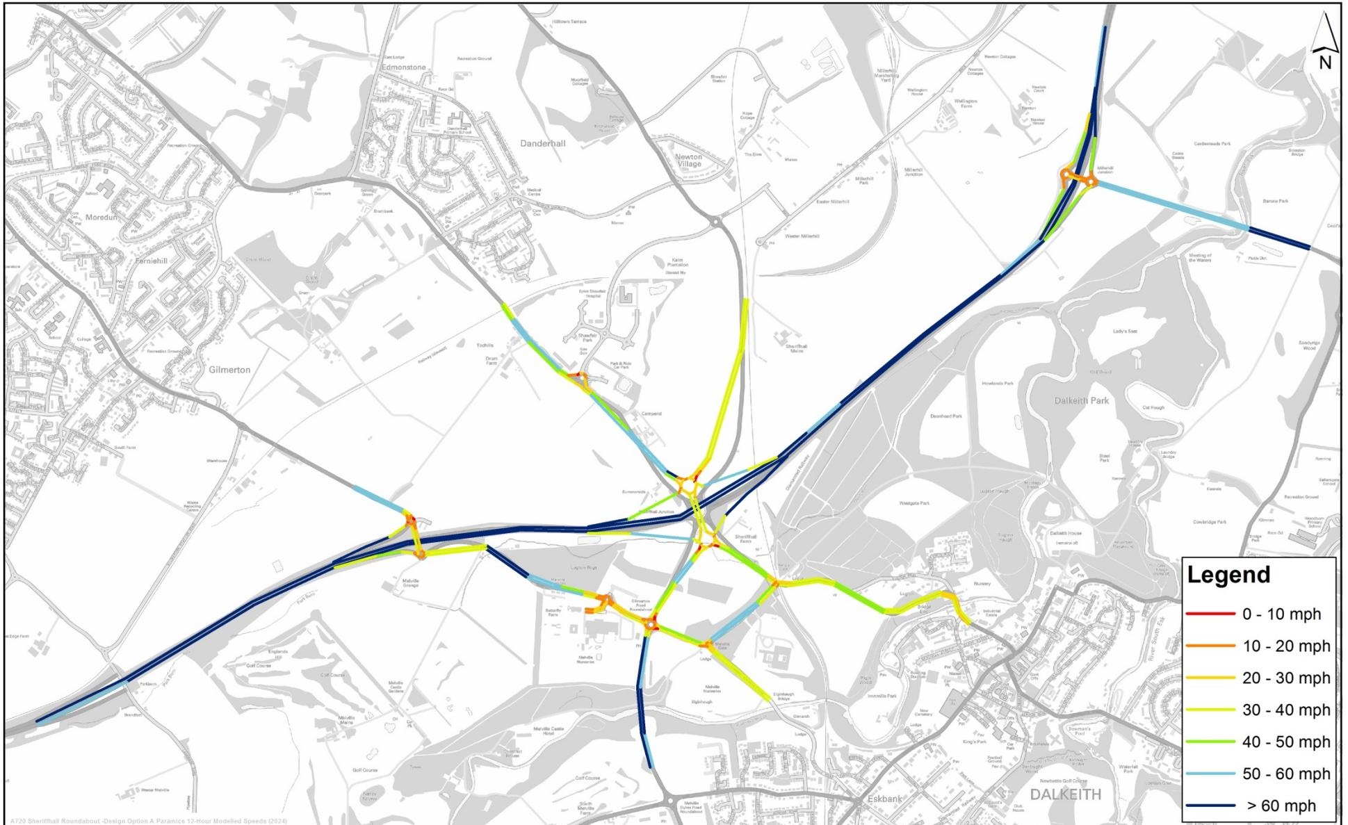
A720 Sheriffhall Roundabout - Design Option A Paramics 12-Hour Modified Speeds (2024)
