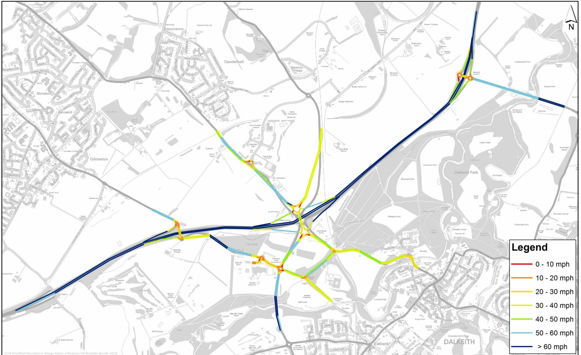
A720 Sheriffhall Roundabout - Design Option A Paramics AM Modelled Speeds (2024)
