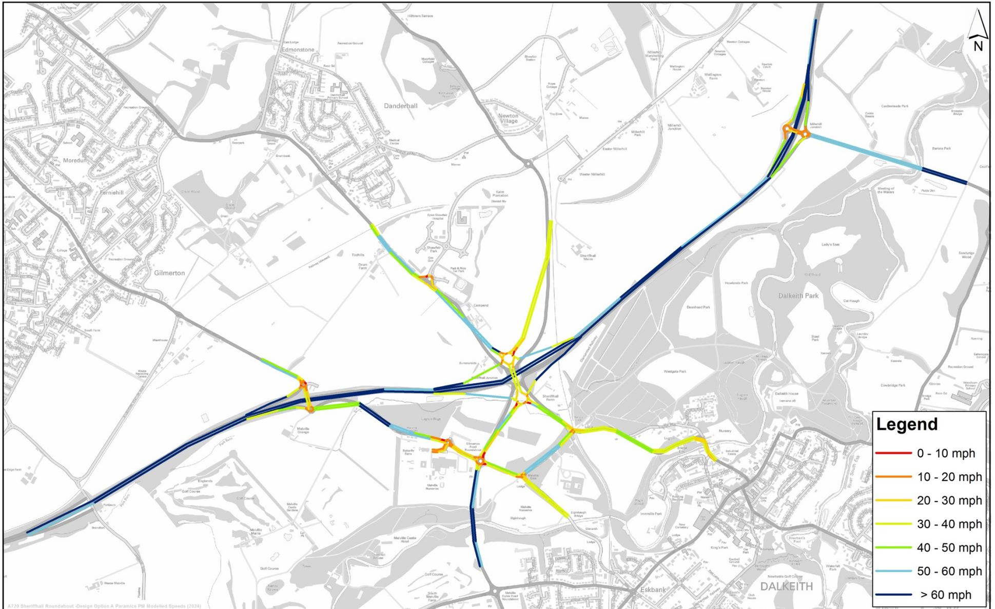
A720 Sheriffhall Roundabout - Design Option A Paramics PM Modelled Speeds (2024)
