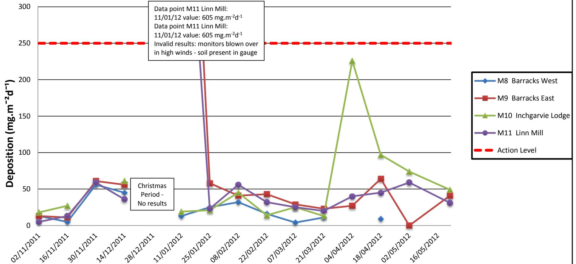
**Note:** Frisbee dust data results missing for Inchgarvie Lodge for 30/11/11 as the bottle was broken in transit. Data is missing for Barracks West for 04/04/12, 02/04/12 and 16/05/12 due to poor accessibility. No Frisbee dust data results were collected on 28/12/11 as this was during the Christmas period, during which no works were conducted.
