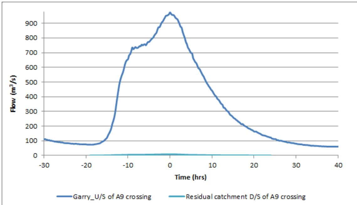
**Hydrology for Hydraulic Model Calibration**
