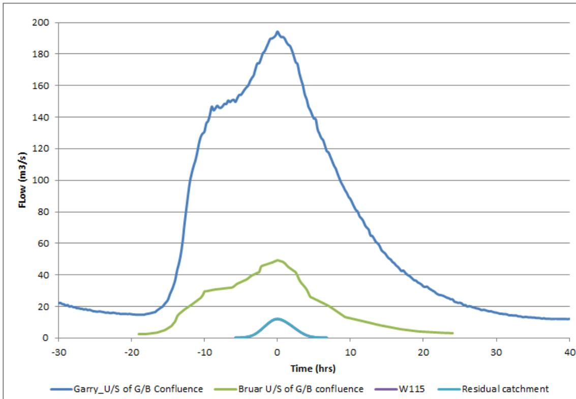
(Note: this arrangement is focused on the design conditions along the tributaries and not the main stem. The flows in the main stem are simply to provide a credible downstream boundary which given the concepts behind what constitutes a design flood event on catchments of differing size will have a rarity that is less than that of the targeted tributary flood).
