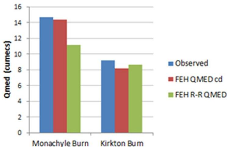
**Diagram 8: Comparison of QMED estimates from the FEH Rainfall-runoff method and the FEH Statistical method to the observed QMED values obtained from observed data in two small mountainous catchments in the Central Highlands.**
