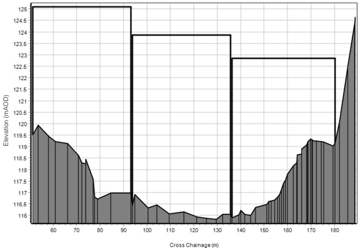
**Diagram 7: Pitaldonich Underbridge 1D schematisation in Flood Modeller**
