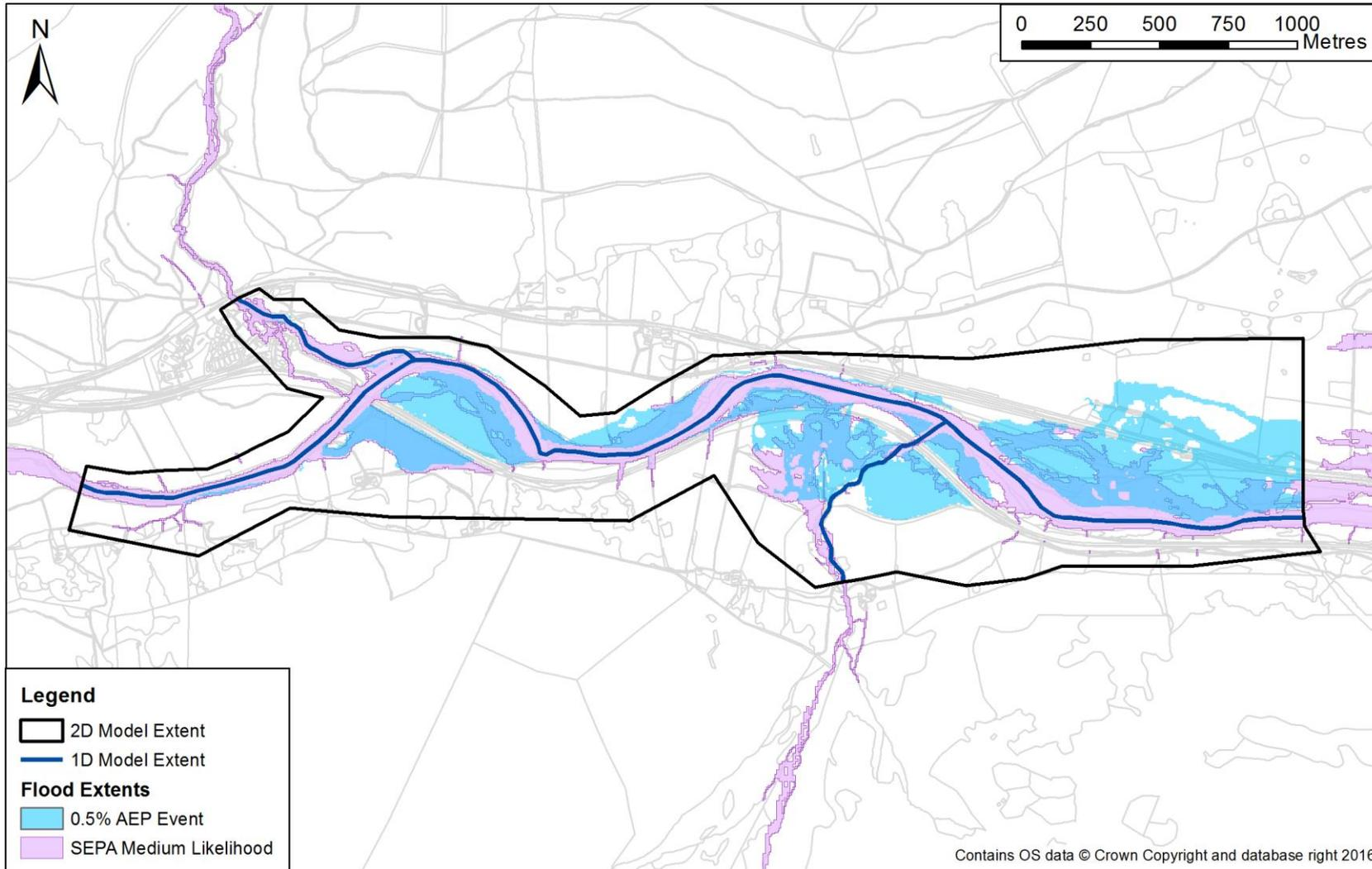
Diagram 23: Model V roughness sensitivity results
