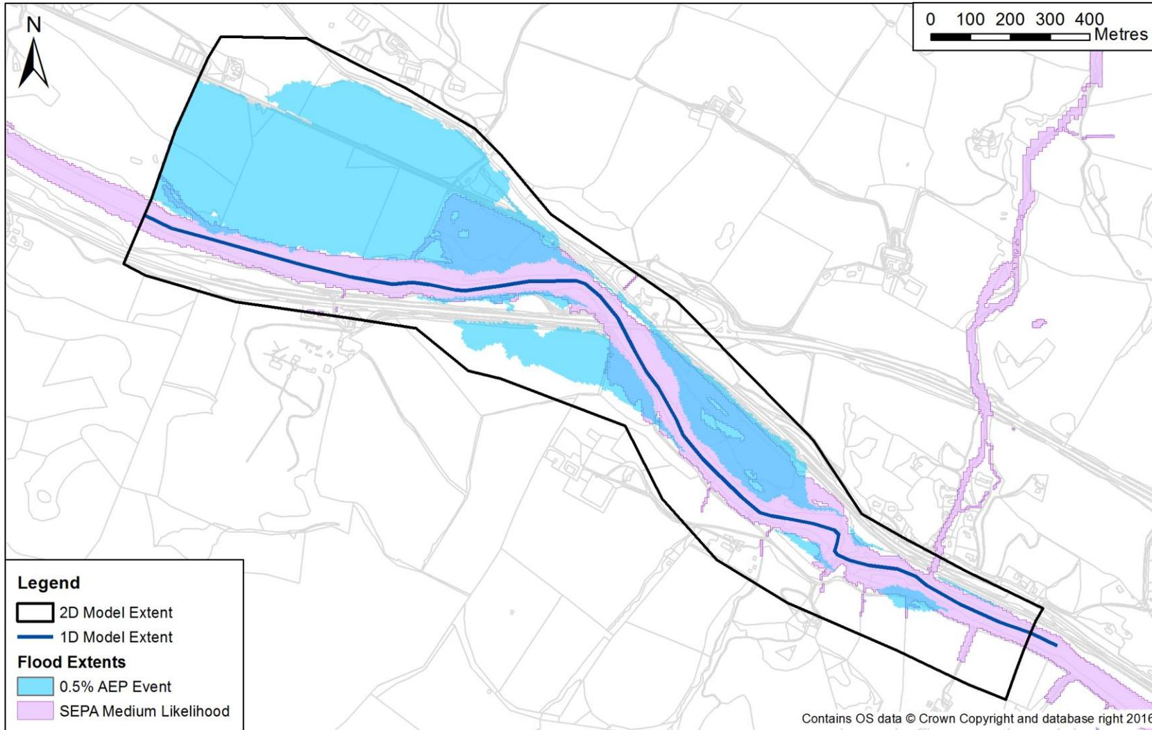
Diagram 22: Model V/VI modelled 0.5% AEP (200-year) flood event extent vs. SEPA medium likelihood fluvial extent
