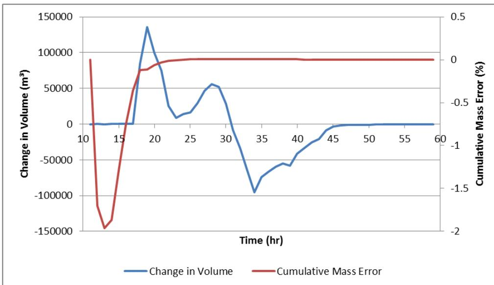
**Diagram 19: Cumulative mass error and change in volume Model VI 0.5% AEP plus CC Event**
