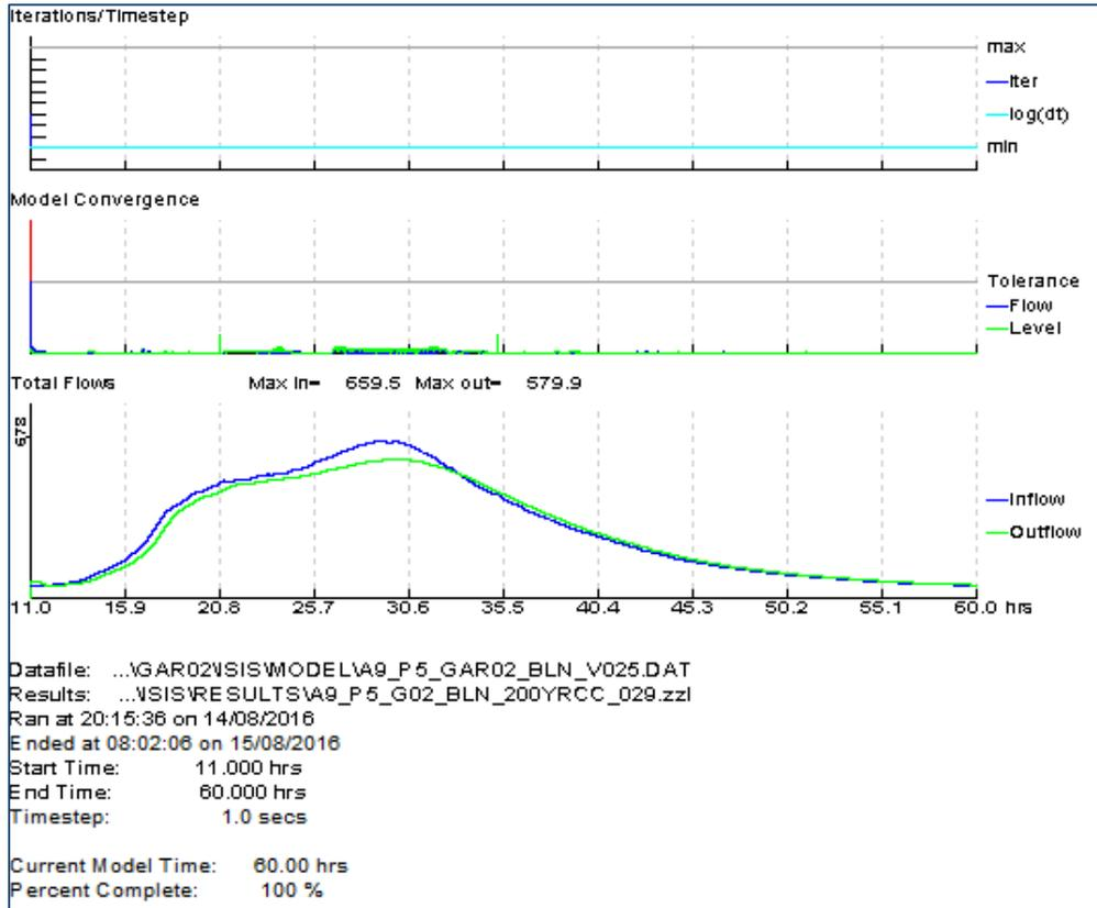
**Diagram 18: Cumulative mass error and change in volume Model V 0.5% AEP plus CC event**
