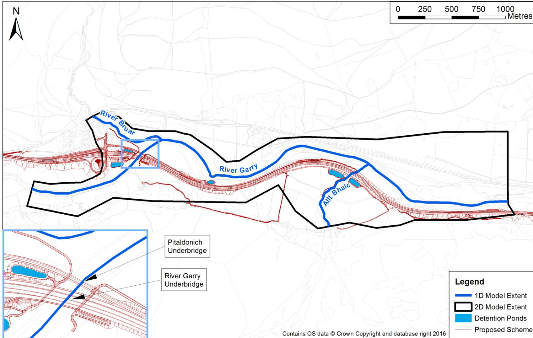
**Diagram 14: River Garry Underbridge proposed scheme design schematisation**
