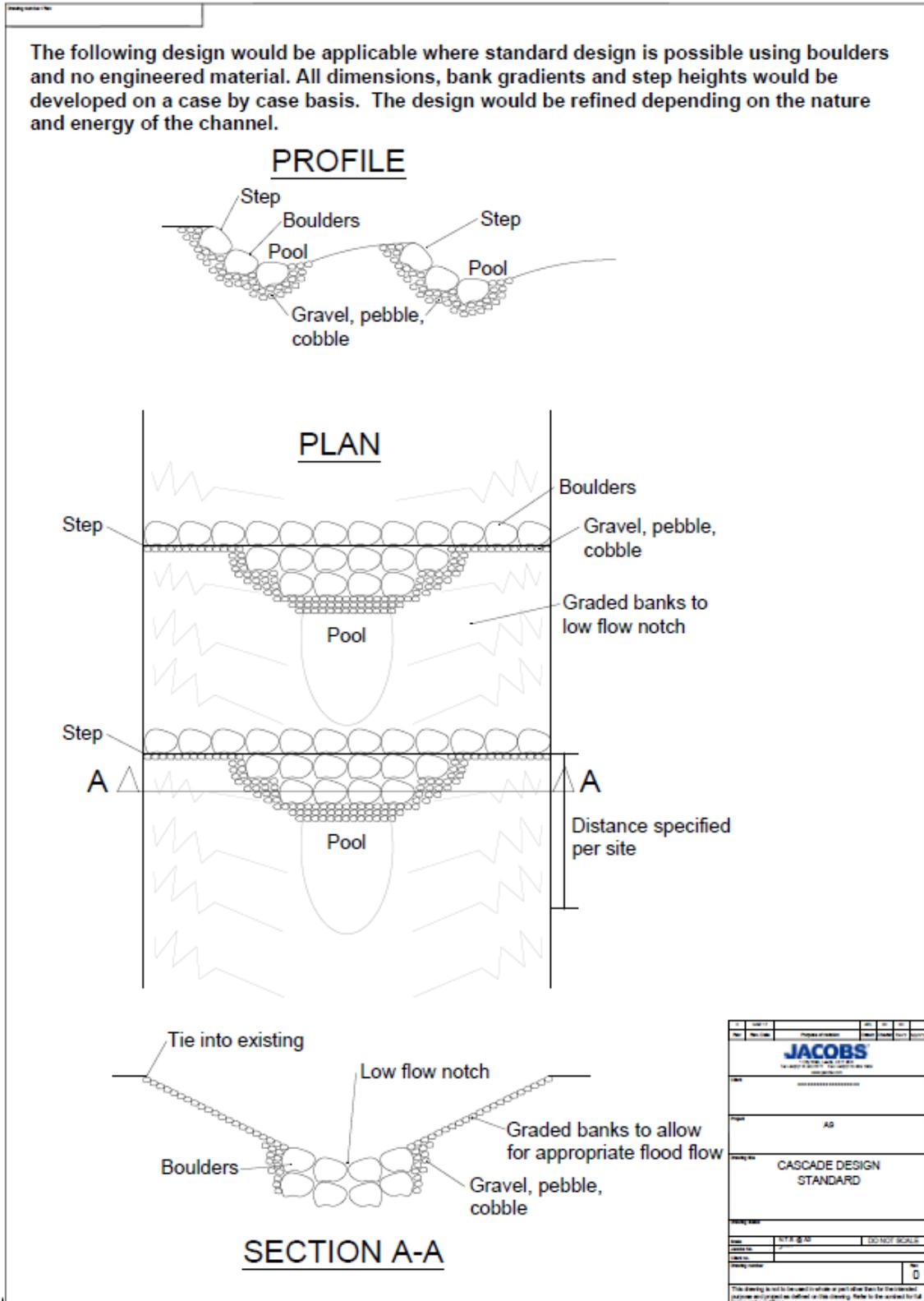
Diagram 4: Conceptual diagram illustrating, in profile, plan view and cross-section, the constituents of a step-pool bed morphology for an over-engineered design for high erosion risk sites
