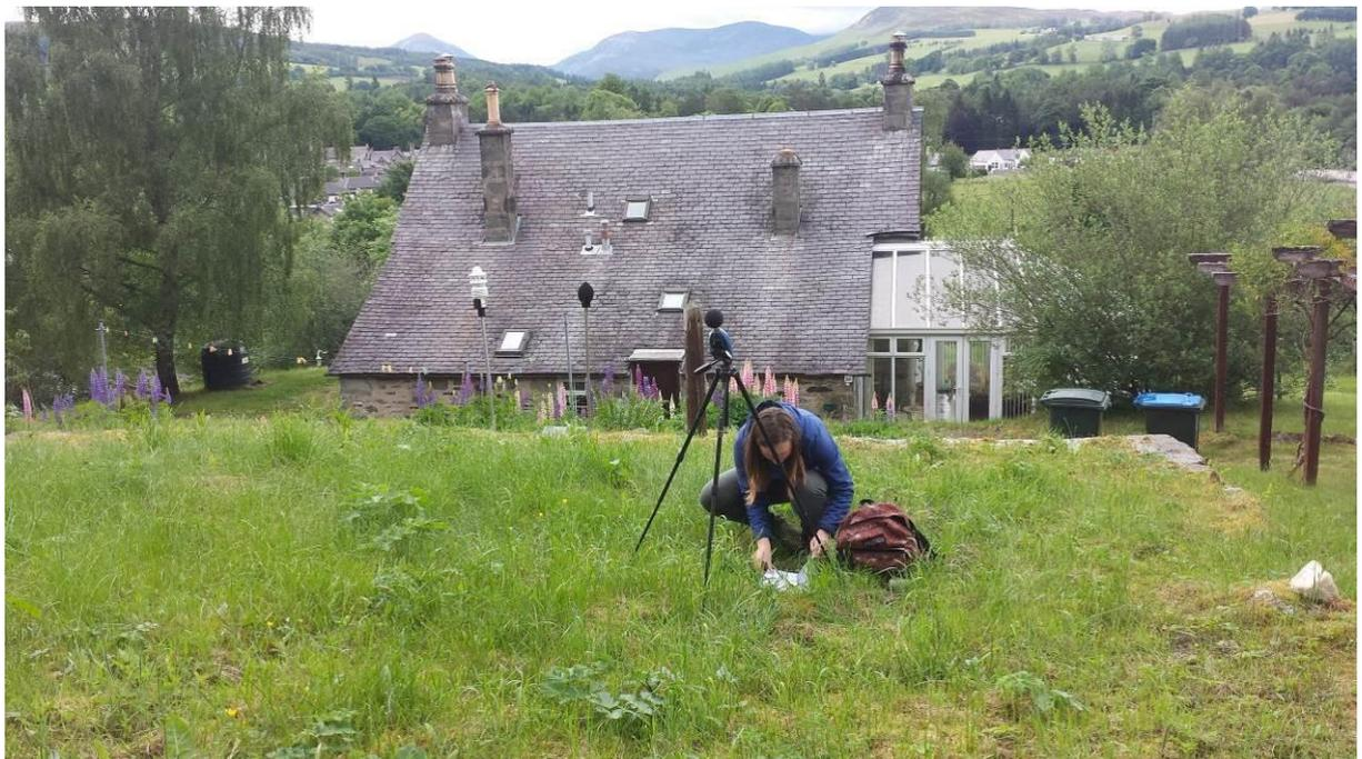
2.1.27 The monitoring equipment was calibrated both before and after the measurement period using a RION NC-74 (s/n 34536108) acoustic calibrator, which has itself been calibrated against a reference set traceable to National and International Standards. There was no significant shift in the observed calibration level.
