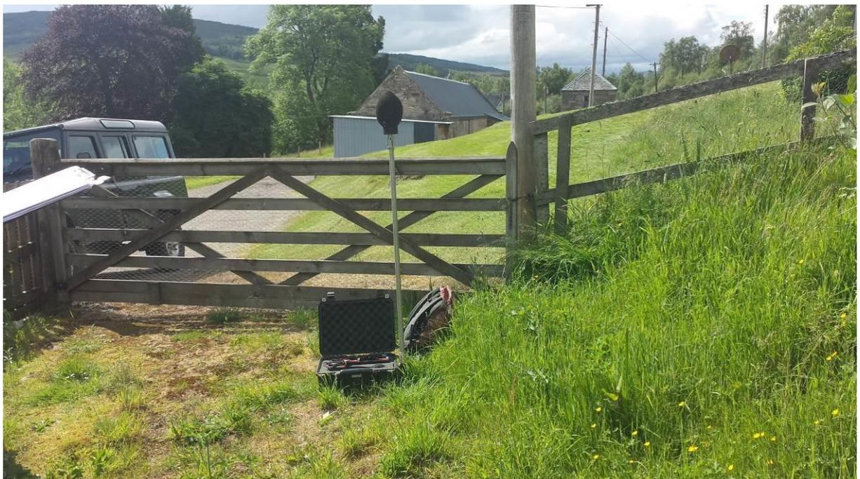
2.1.57 The monitoring equipment was calibrated both before and after the measurement period using a Rion NC-74 (s/n 34536108) acoustic calibrator, which has itself been calibrated against a reference set traceable to National and International Standards. There was no significant shift in the observed calibration level.
