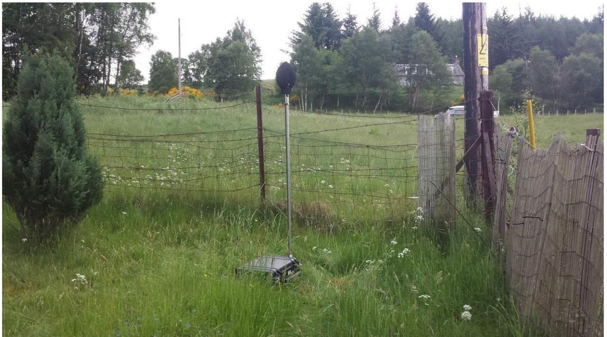
2.1.51 The monitoring equipment was calibrated both before and after the measurement period using a Rion NC-74 (s/n 34536108) acoustic calibrator, which has itself been calibrated against a reference set traceable to National and International Standards. There was no significant shift in the observed calibration level.
