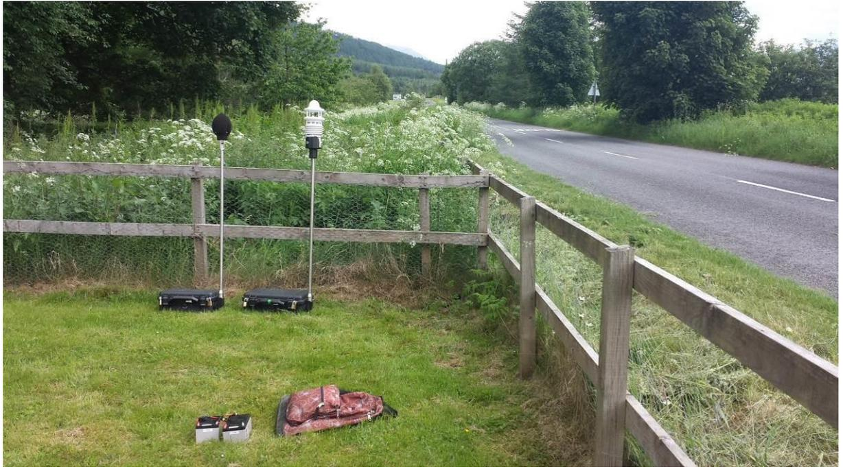
2.1.45 The monitoring equipment was calibrated both before and after the measurement period using a Rion NC-74 (s/n 34536108) acoustic calibrator, which has itself been calibrated against a reference set traceable to National and International Standards. There was no significant shift in the observed calibration level.
