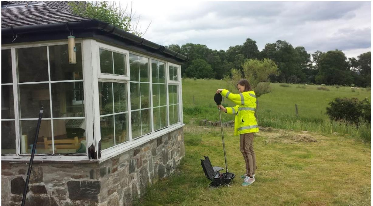
2.1.39 The monitoring equipment was calibrated both before and after the measurement period using a Rion NC-74 (s/n 34536108) acoustic calibrator, which has itself been calibrated against a reference set traceable to National and International Standards. There was no significant shift in the observed calibration level.
