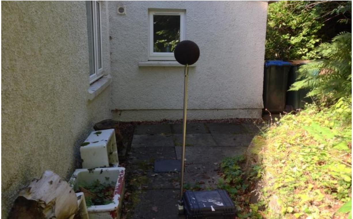
2.8.2 The monitoring equipment was calibrated both before and after the measurement period using an acoustic calibrator (s/n 00830793), which has itself been calibrated against a reference set traceable to National and International Standards. There was no significant shift in the observed calibration level.
