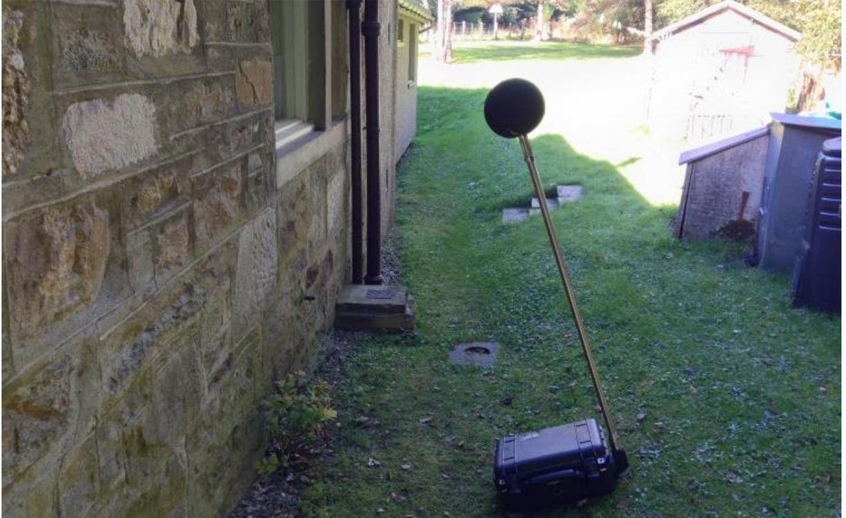
2.7.2 The monitoring equipment was calibrated both before and after the measurement period using an acoustic calibrator (s/n 00830793), which has itself been calibrated against a reference set traceable to National and International Standards. There was no significant shift in the observed calibration level.
