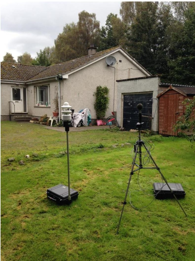
2.3.2 The monitoring equipment was calibrated both before and after the measurement period using an acoustic calibrator (s/n 00830793), which has itself been calibrated against a reference set traceable to National and International Standards. There was no significant shift in the observed calibration level.
