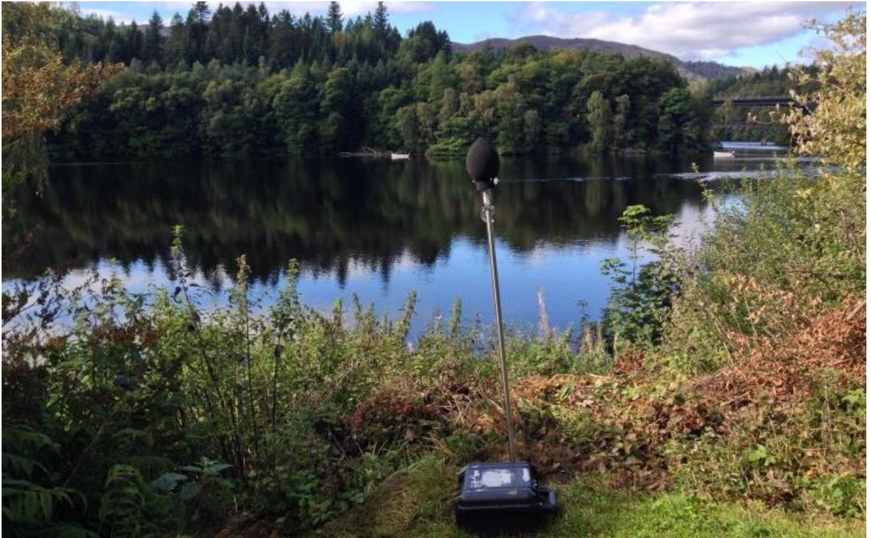
2.6.2 The monitoring equipment was calibrated both before and after the measurement period using an acoustic calibrator (s/n 00830793), which has itself been calibrated against a reference set traceable to National and International Standards. There was no significant shift in the observed calibration level.
