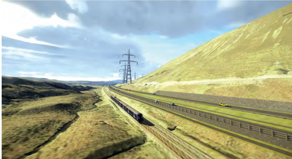
Figure 2-4: Proposed split-level carriageways through Pass of Drumochter
