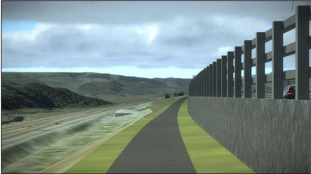
Figure 9.1: The retaining wall and barrier forms a boundary to NMU1 (NCN7)
