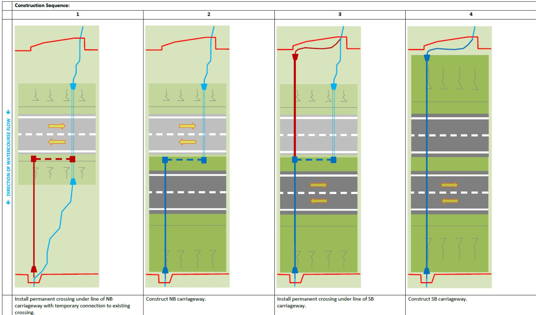
Figure 8: Widening to the west – road on embankment – off-line watercourse alignment
