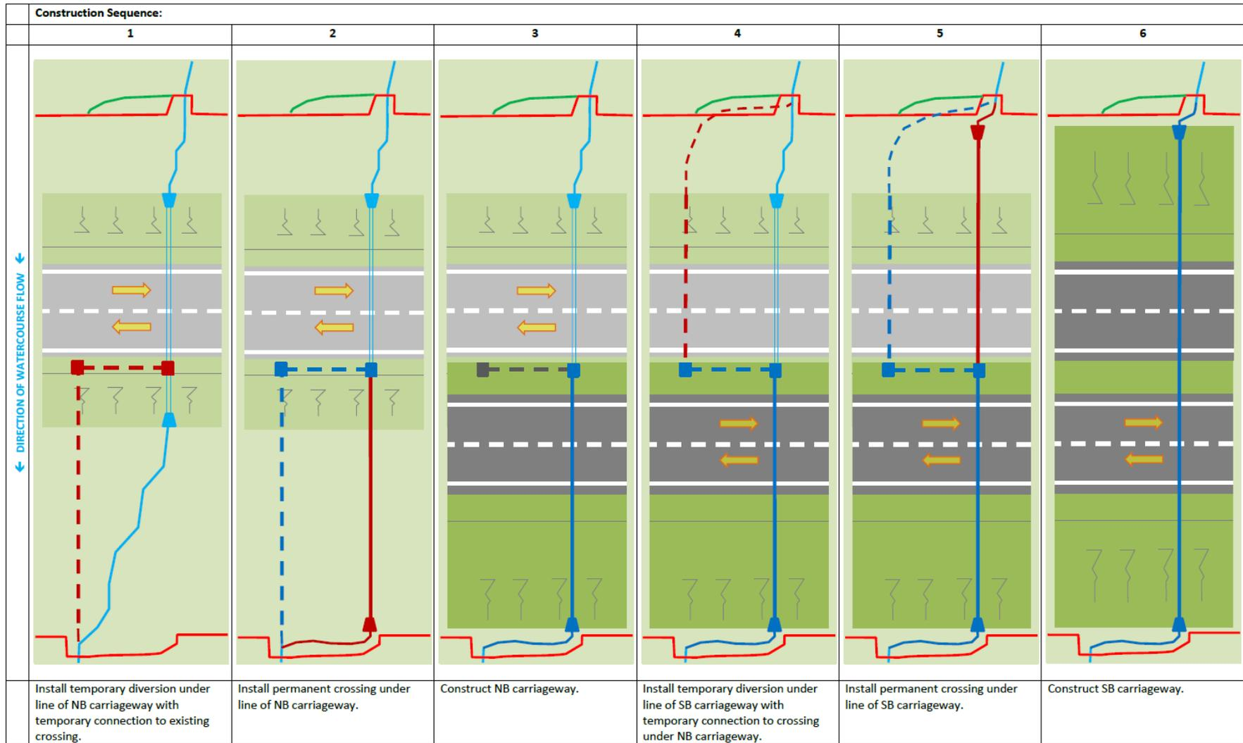
Figure 9: Widening to the west – road on embankment – on-line watercourse alignment
