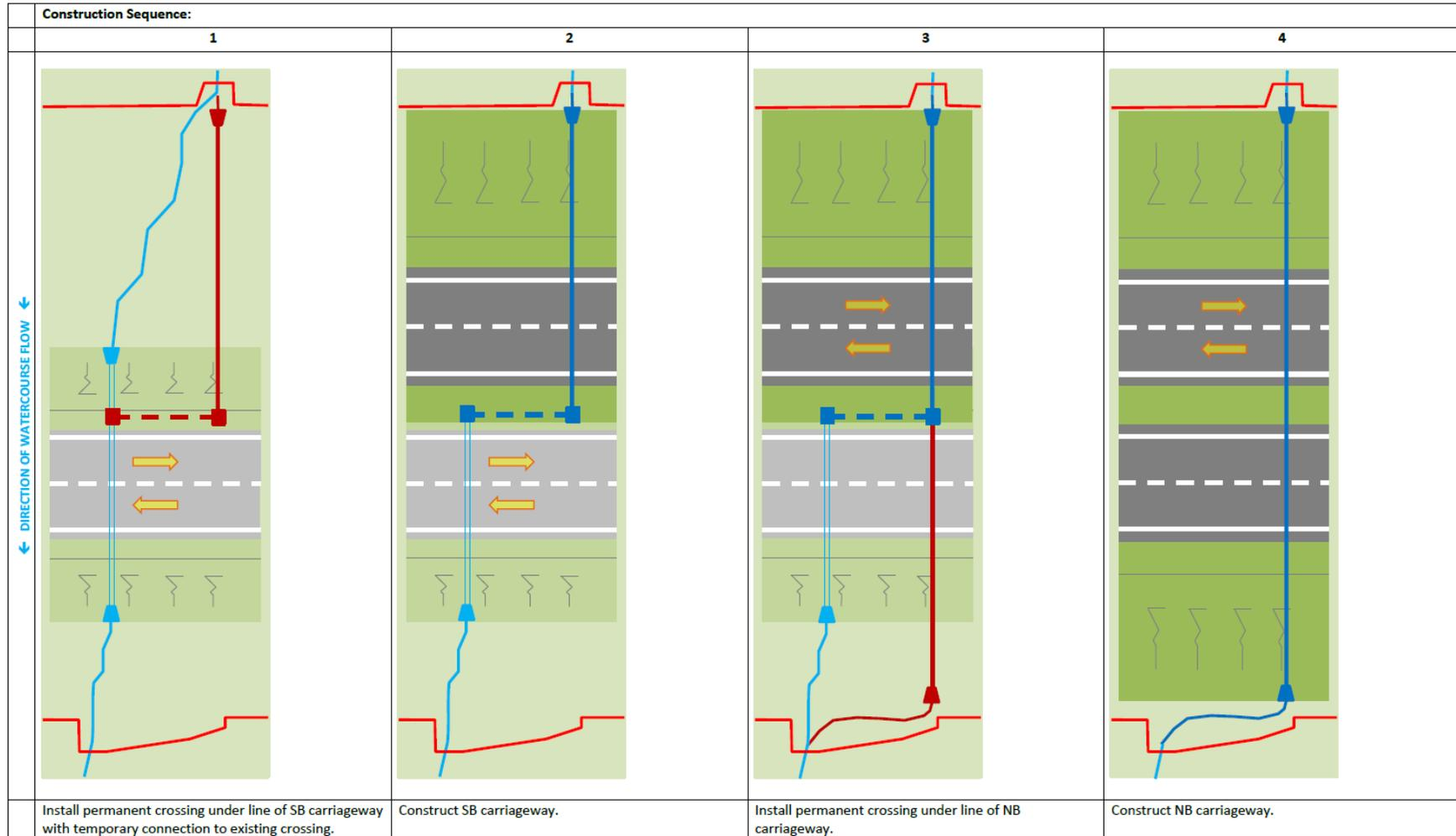
Figure 6: Widening to the east – road on embankment – off-line watercourse alignment
