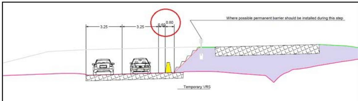
Figure 1: Proposed cross section showing construction of southbound carriageway
