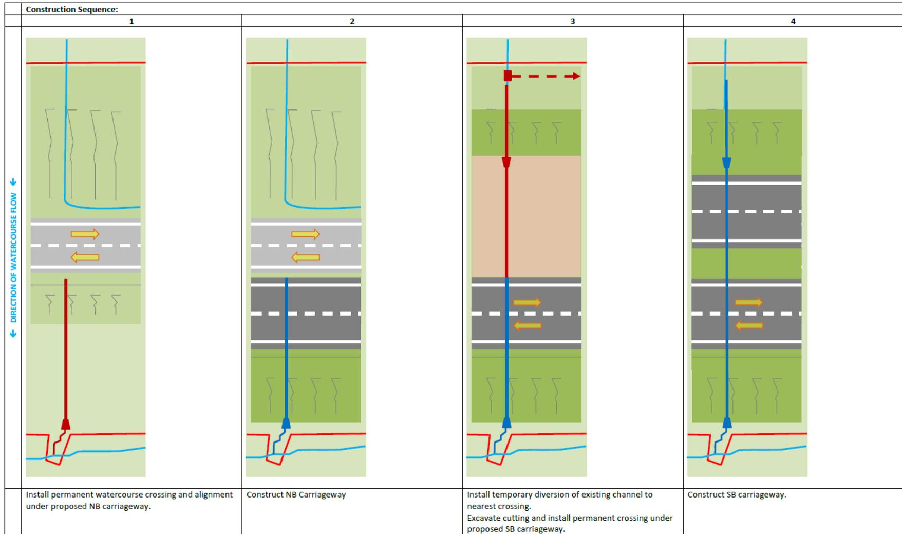
Figure 13: New watercourse crossing – widening to the east (road in cutting) and widening to the west (road in embankment)
