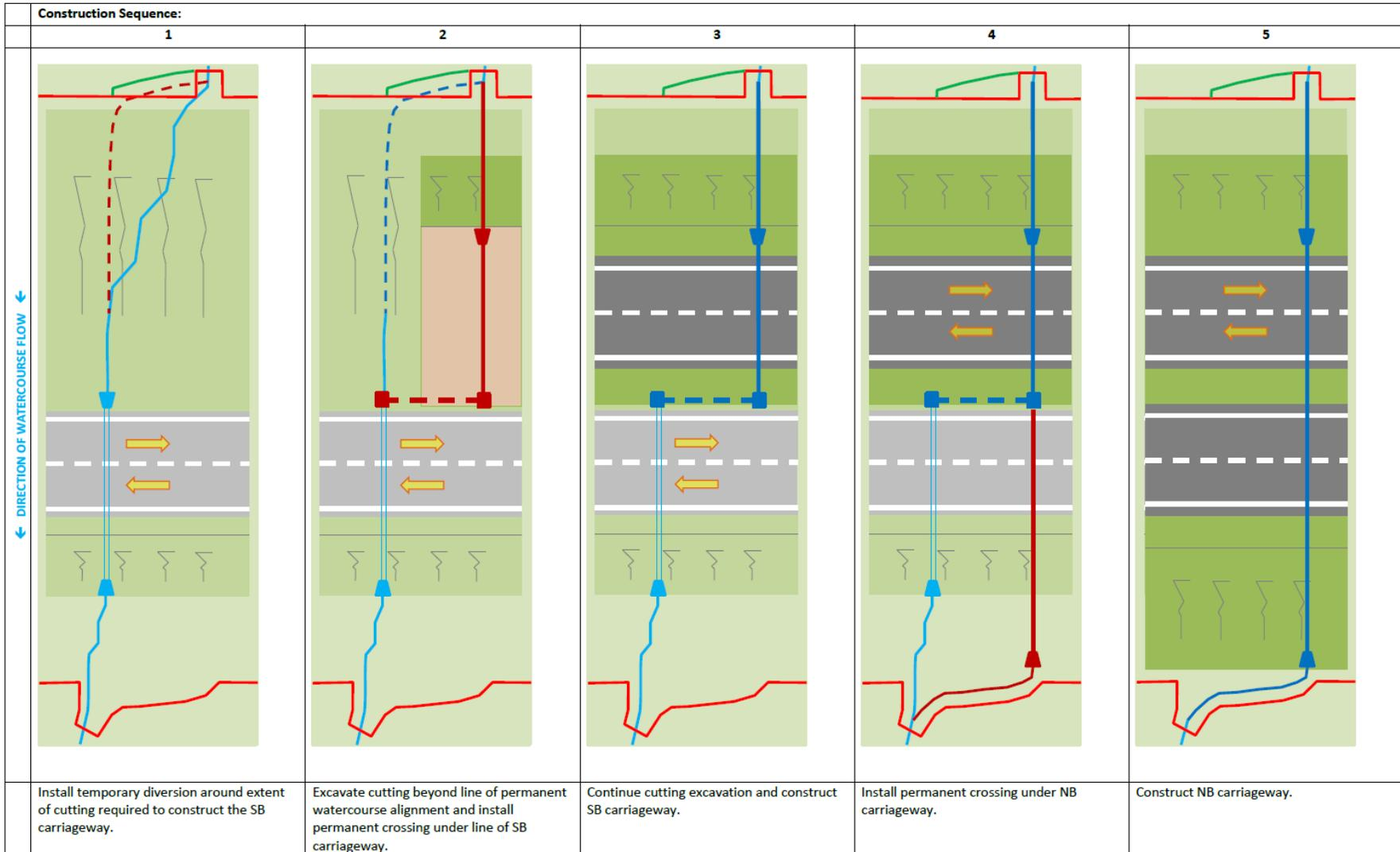
Figure 10: Widening to the east – road in cutting – off-line watercourse alignment
