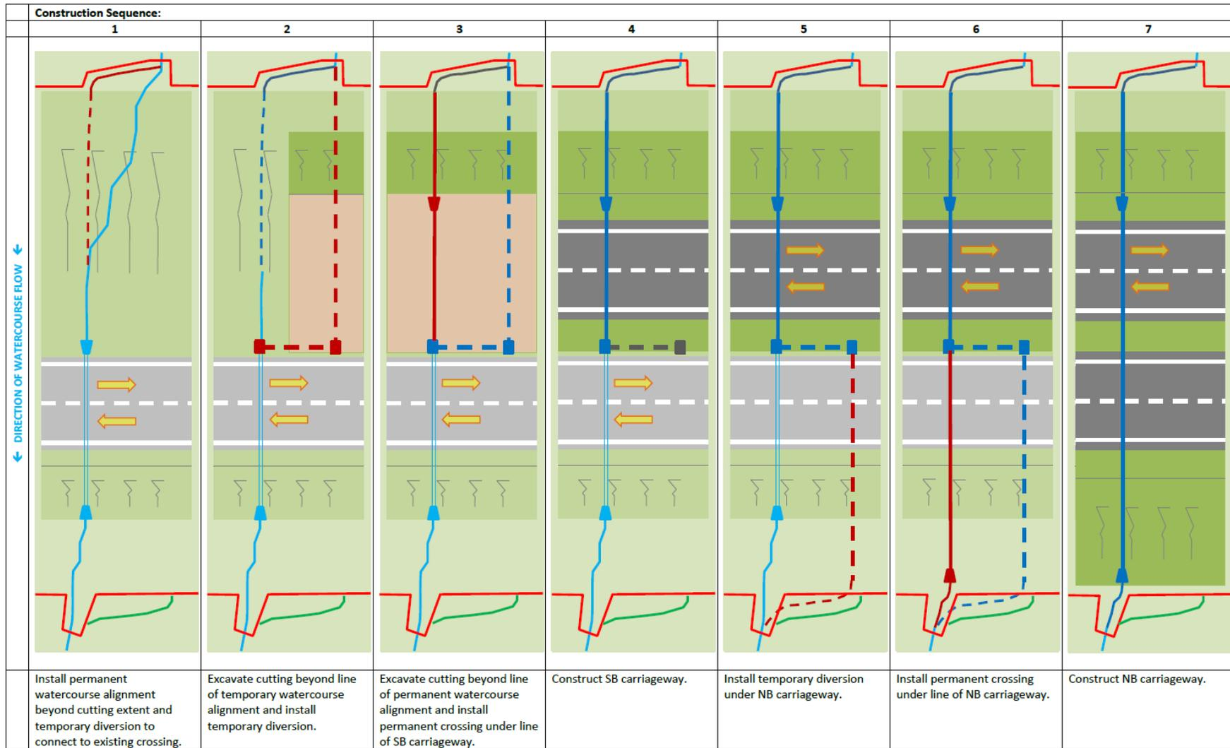
Figure 11: Widening to the east – road in cutting – on-line watercourse alignment
