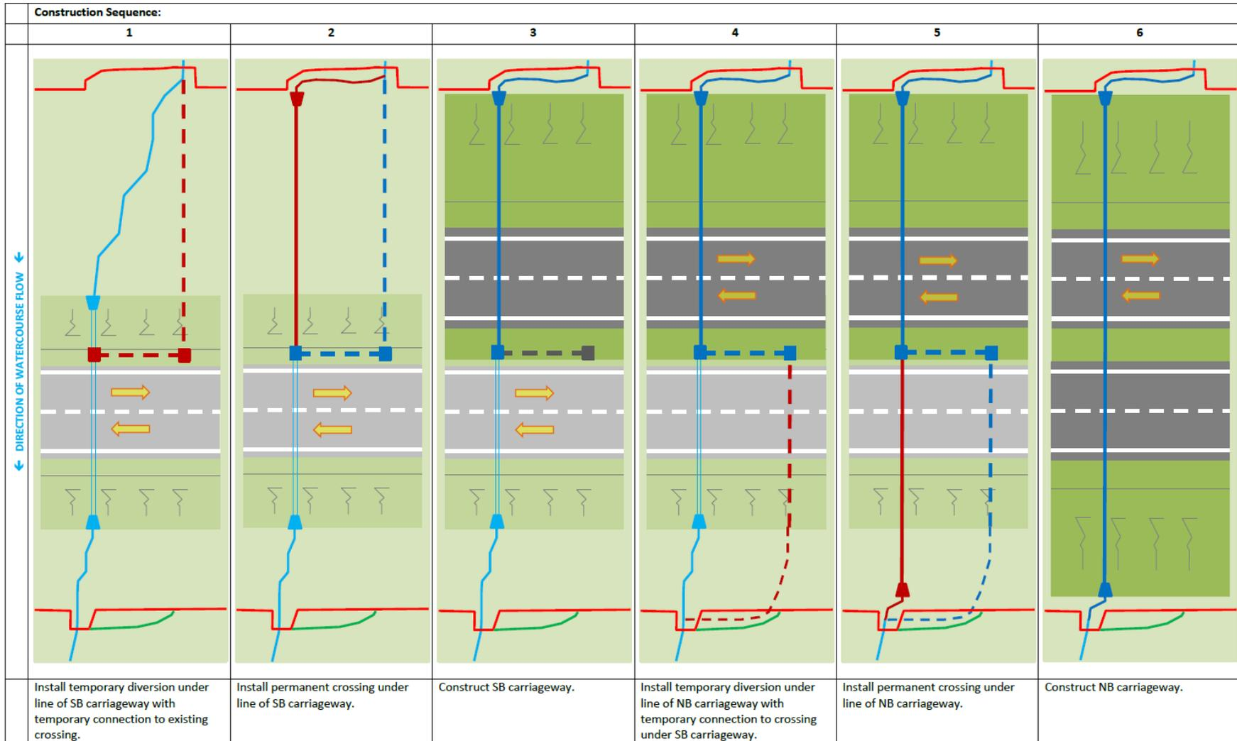
Figure 7: Widening to the east – road on embankment – on-line watercourse alignment
