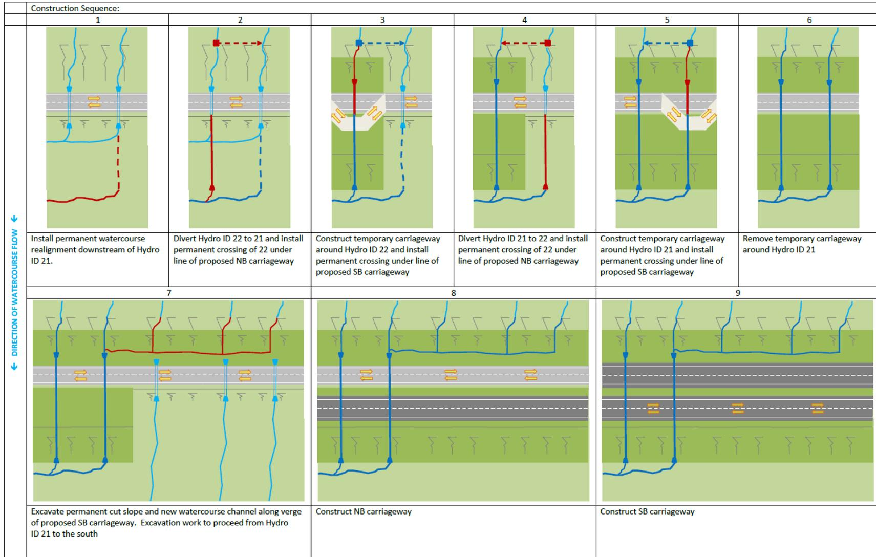
Figure 12: On-line watercourse alignment – widening to the east (road in cutting) and widening to the west (road on embankment)
