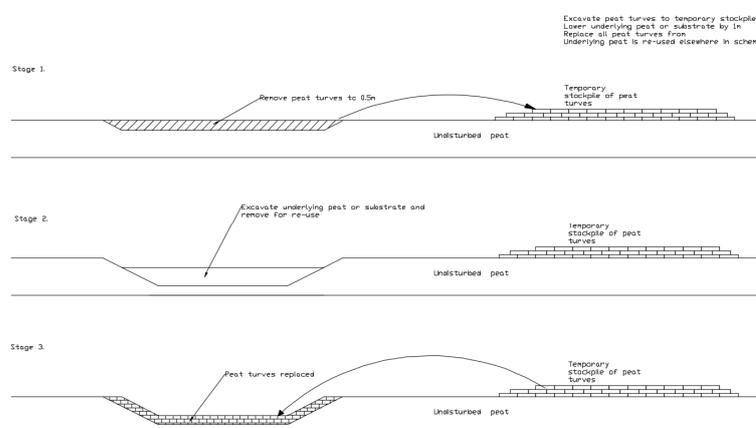
Figure 5: Calculation of Excavation and Re-instatement Volumes (Compensatory Flood Storage)
