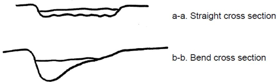
Figure 26: Example cross sections for plane- riffle channels
