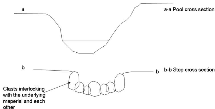
Figure 19: Example cross sections for a step- pool channel
