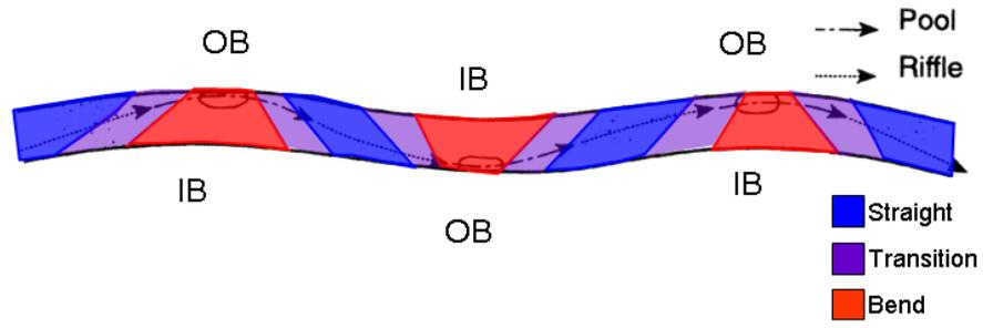
Figure 27: Example locations of plane- riffle cross sections
