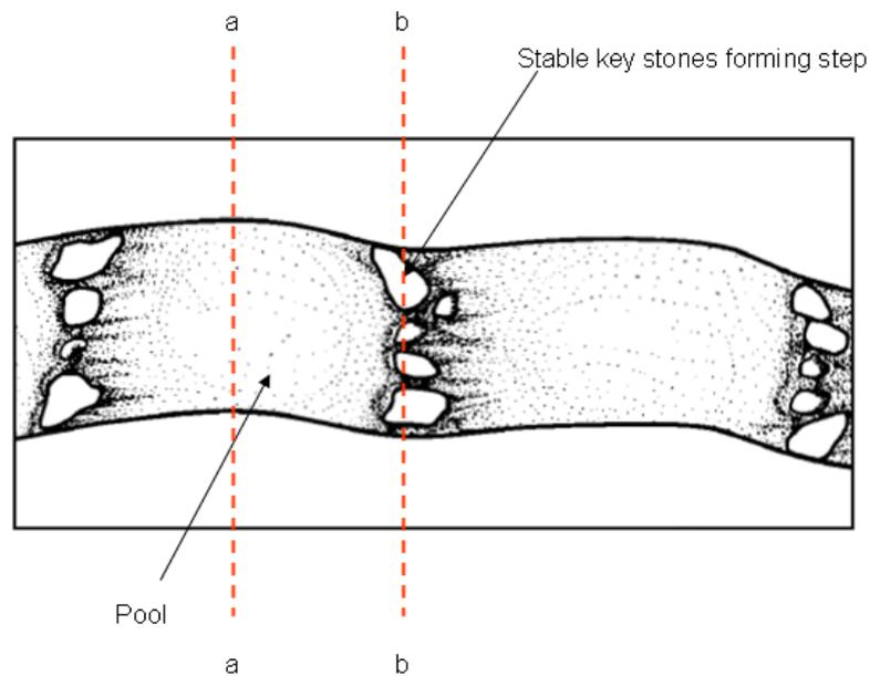
Figure 18: Example planform for a step –pool channel (based on Montgomery and Buffington, 1997)
