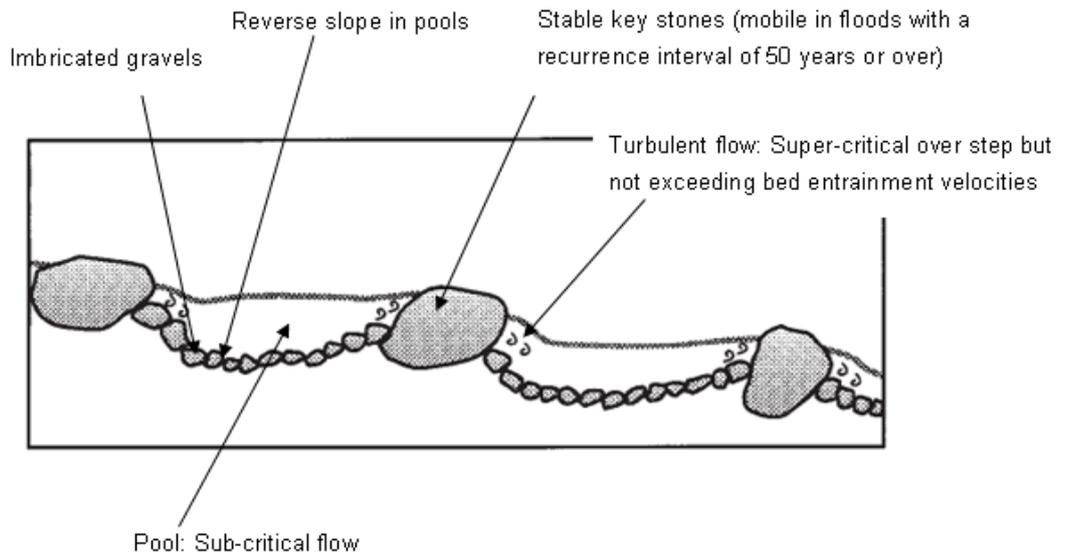
Figure 17: Example long profile of step –pool channel (based on Montgomery and Buffington, 1997)
