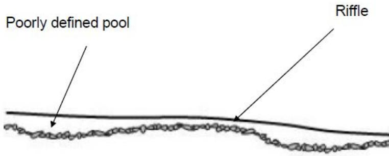
Figure 24: Example long profile of a plane – riffle channel (SEPA, 2011)
