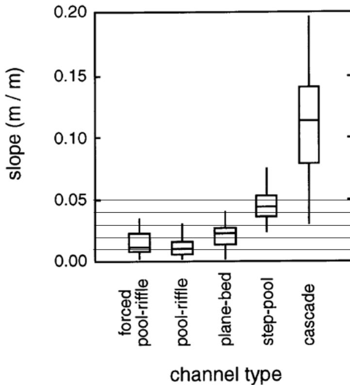
Figure 12: Slope distribution for different channel reaches (Montgomery and Buffington, 1997)
