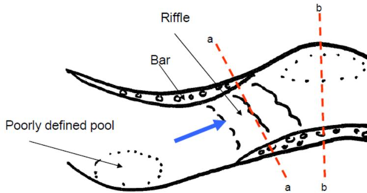
Figure 25: Example planform of a plane – riffle channel
