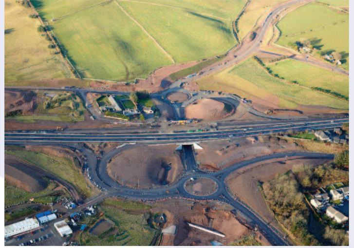
**Balmedie Underpass:** The new underpass can be clearly seen with the new roundabouts and access roads approaching completion.
