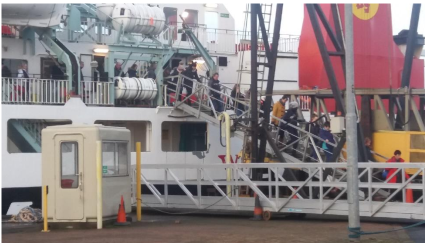
Photo 1. The gangway at Ardrossan showing a 45° angle, which is extremely difficult for disabled travellers to negotiate.
